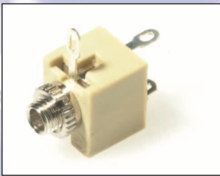
JYO-25 mono switched 2.5mm Jack Socket. Panel mounting with solder tags. Supplied with ring nut.
