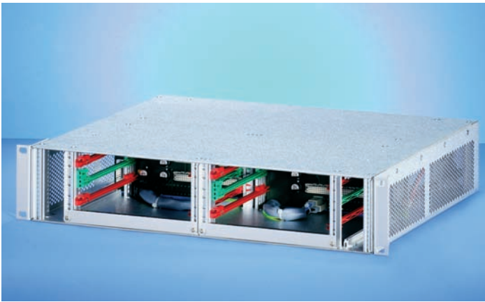
Application: 2 U version with 2 x 3 U assembly
