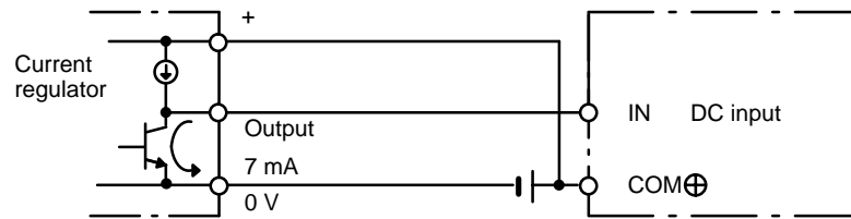
NPN open-collector output
