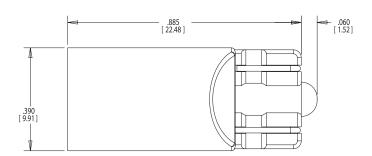
Measurements are typical Dimensions are inches [mm]
