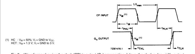
Fig.6 Waveforms showing the clock (CP) to output (Q<sub>n</sub>) propagation delays, the clock pulse width, output transition times and the maximum clock pulse frequency.
