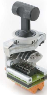
Lever switch, 2-5 positions, cage clamp®, aluminium bezel, silver contacts, 33.5mm mounting
