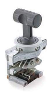
Lever switch, 2-5 positions, plug-in or screw terminals, aluminium bezel, silver contacts with positive opening, 33.5mm mounting
