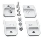
Bracket is molded from fiberglass reinforced polyester. Kit includes four brackets, hardware and installation instructions. Mounting hole dimensions with mounting brackets installed are: [G + 2.50 (64 mm)] x [H + .50 (13 mm)] See Screw- or Hinged-Cover with Quick-Release Latch, Type 4X tables for G and H dimensions.
