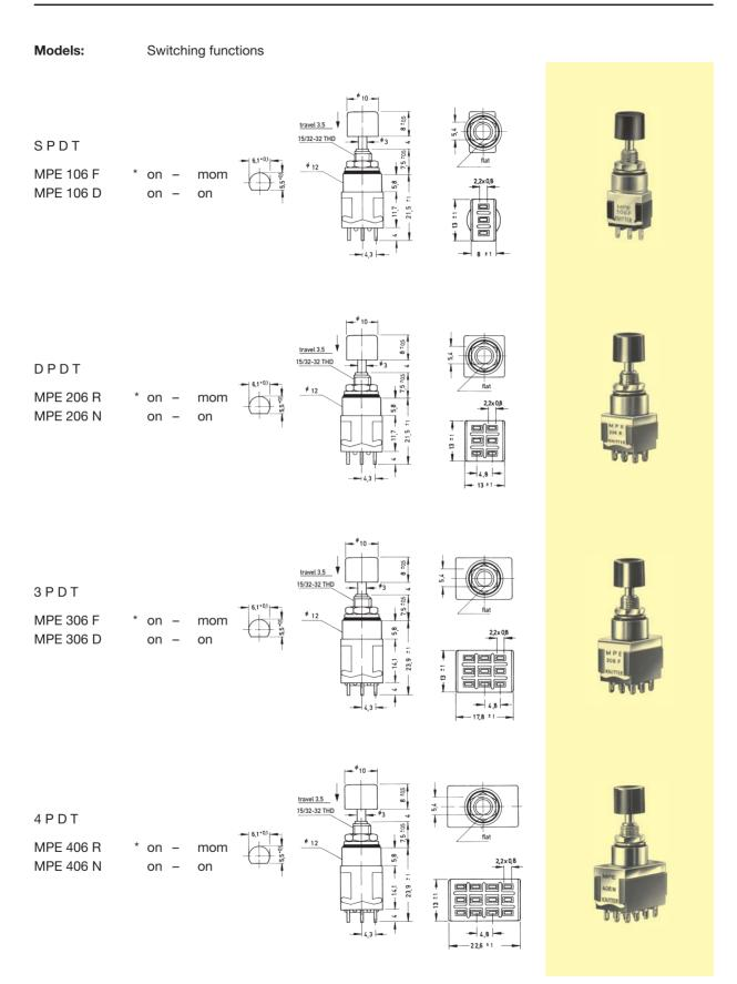
$<sup>^{\</sup>star}$  When looking at the brand name the normally closed contact is on the right-hand side.
