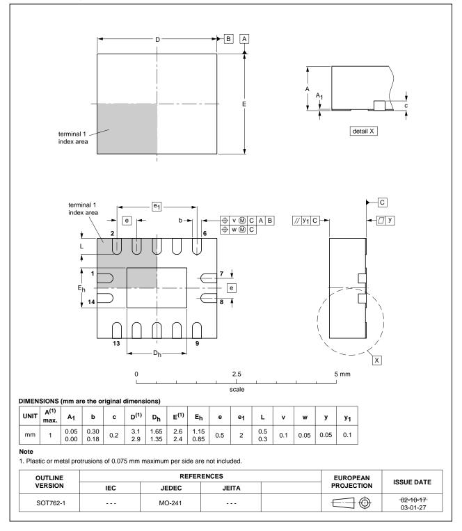
DHVQFN14: plastic dual in-line compatible thermal enhanced very thin quad flat package; no leads; 14 terminals; body 2.5 x 3 x 0.85 mm SOT762-1
