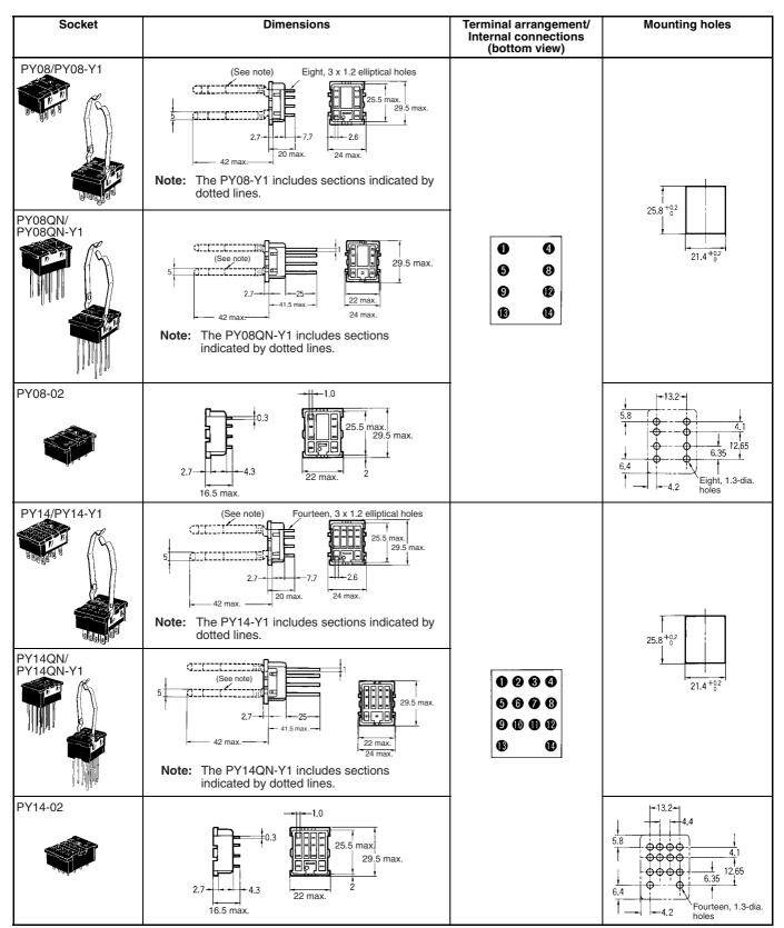
Note: Use a panel with plate thickness of 1 to 2 mm for mounting the Sockets.
