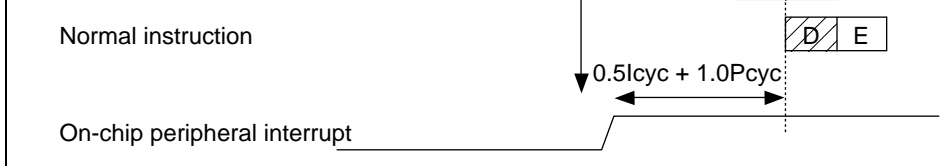
Figure 5.14 Pipeline Operation when Interrupts are Enabled by Means of SR M
