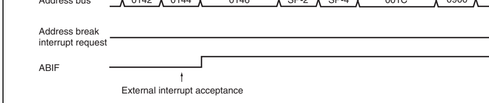
Figure 4.4 Operation when Another Interrupt is Accepted at Address Break Set Instruction
