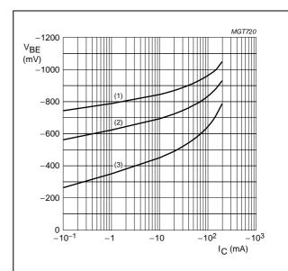
BC857C;  $V_{CE} = -5 \text{ V}.$
