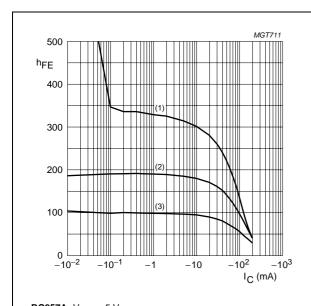
BC857A;  $V_{CE} = -5 \text{ V}.$
