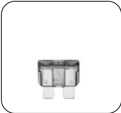
ATC® Blade-Type Fuse Fast Acting Voltage Rating: 32V DC Interrupting Rating: 1,000A Agency Information: UL Recognized, (3-40A) (Guide JFHR2, File E56412)
