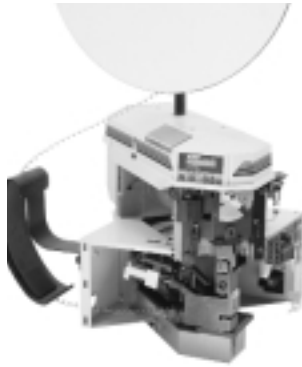
Model G Splice Terminating Machine, P/N 356462-2 & Applicator
