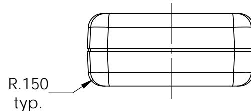
Enclosure can hold either a 0.032" PCB or a 0.063 PCB
