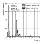
\*1. The tests were conducted at an ambient temperature of 23°C.
