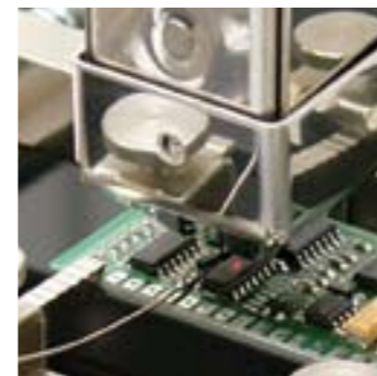
Temperature-controlled SMD soldering
