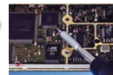
DIG20A45 with Chip Tool and ERSA RESISTRONIC control system. 422 desoldering tip series see page 41
