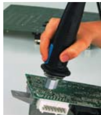
High-mass through-hole desoldering
