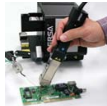
Rapid, simple and safe hand-held component removal
