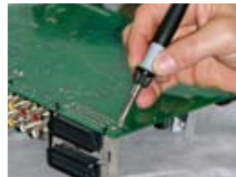
High-mass through-hole soldering with the i-Tool
