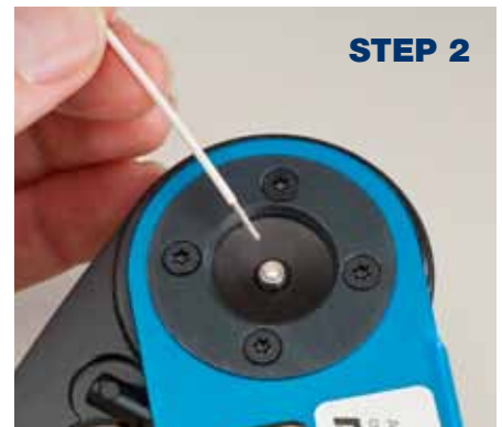
INSERT PRE-STRIPPED WIRE
