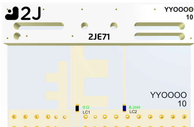
3D View of matching components and recommended values (LC1=0 Ohm, LC2=8.2nH)
