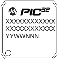
100-Lead TQFP (14x14x1 mm)
