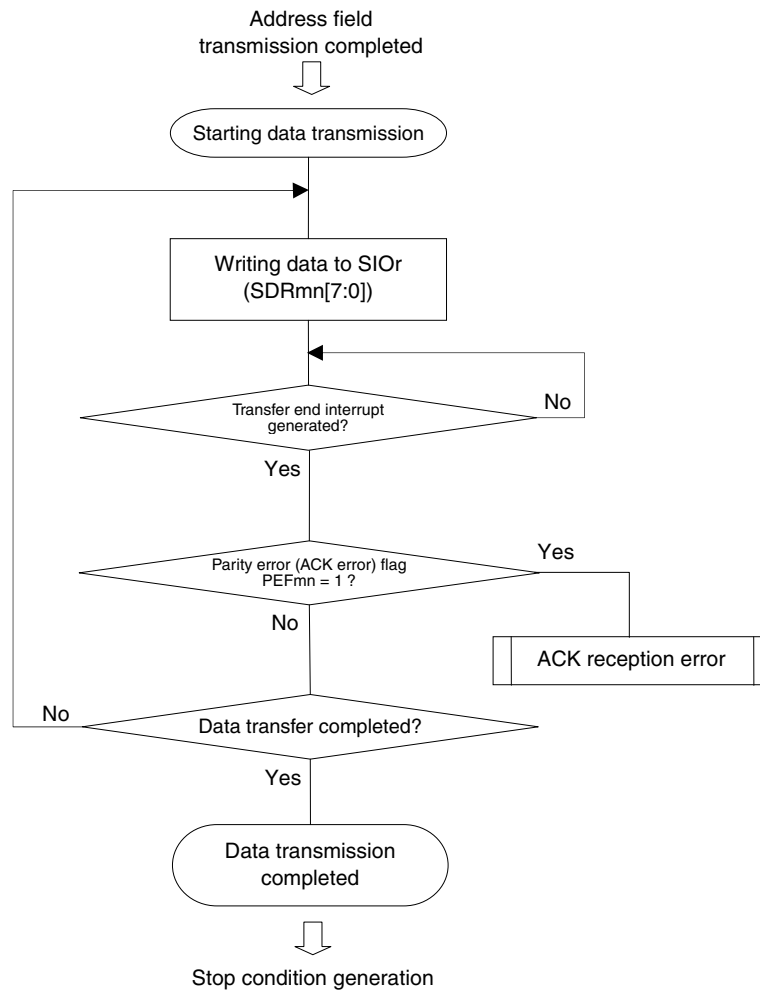
Figure 12-111. Flowchart of Data Transmission
