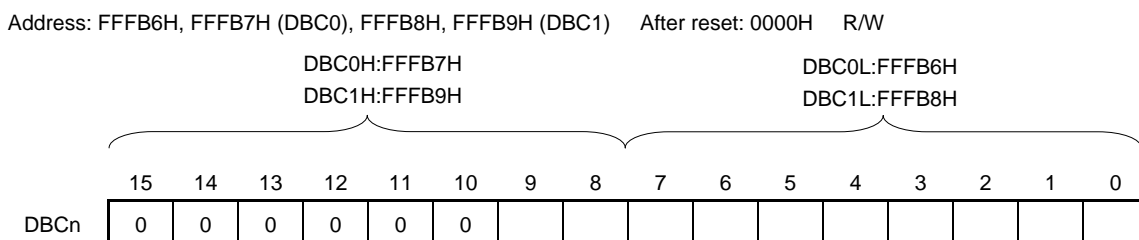
Figure 14-3. Format of DMA Byte Count Register n (DBCn)
