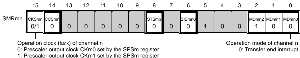
Figure 11-99. Example of Contents of Registers for Address Field Transmission of Simplified I 2 C (IIC00, IIC01, IIC11, IIC20)
