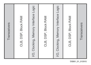
Figure 1: Device with Columnar Resources
