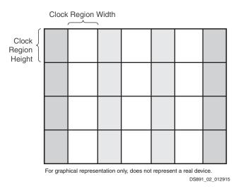
Figure 2: Column-Based Device Divided into Clock Regions
