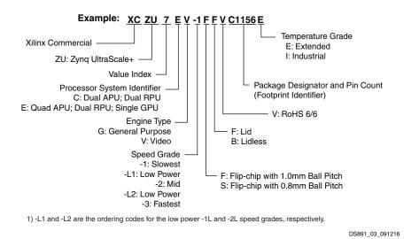
Figure 3: Zynq UltraScale+ MPSoC Ordering Information
