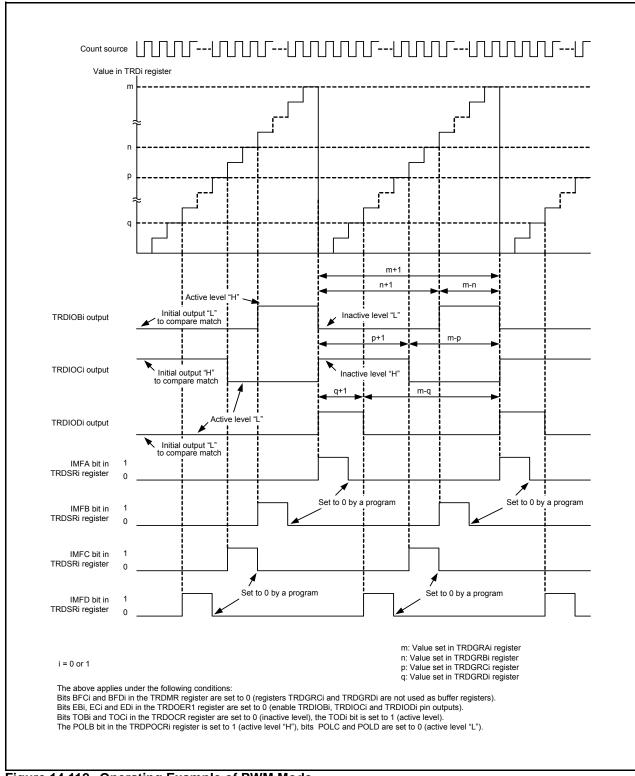
Figure 14.112 Operating Example of PWM Mode
