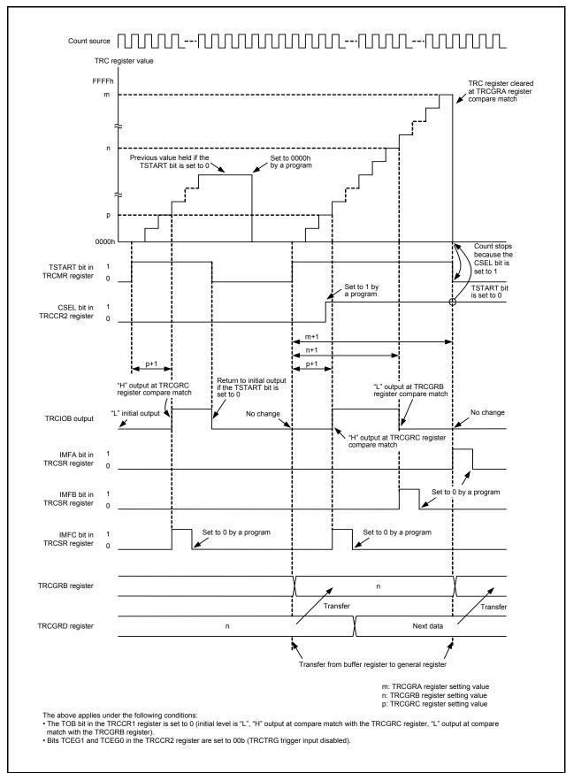
Figure 14.58 Operating Example of PWM2 Mode (TRCTRG Trigger Input Disabled)
