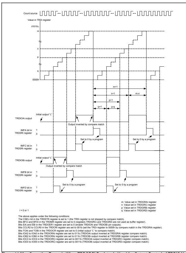
Figure 14.99 Operating Example When TRDGRCi Register is Used for Output Control of TRDIOAi
