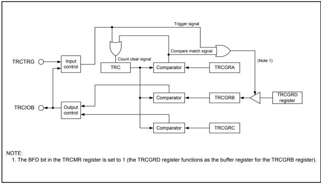
Figure 14.56 Block Diagram of PWM2 Mode
