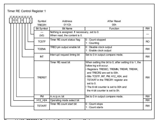
Figure 14.169 TRECR1 Register in Output Compare Mode
