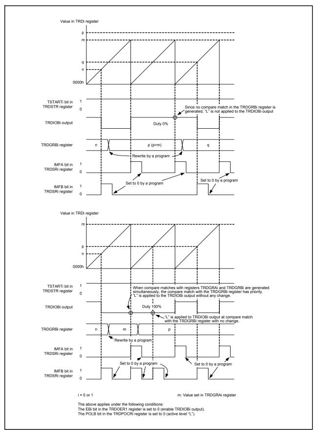
Figure 14.113 Operating Example of PWM Mode (Duty 0%, Duty 100%)
