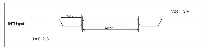
External Interrupt INTi Input Timing Diagram when Vcc = 3 V Figure 21.17
