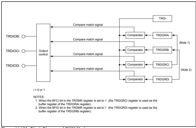
Figure 14.100 Block Diagram of PWM Mode
