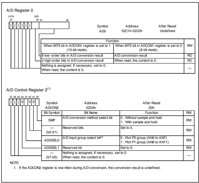
Figure 18.2 **Registers AD0 and ADCON2**
