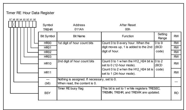
Figure 14.159 TREHR Register in Real-Time Clock Mode
