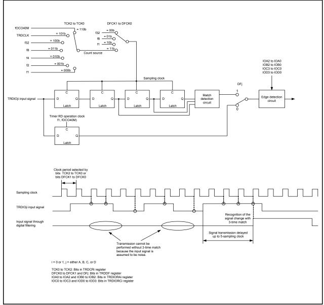
Figure 14.82 Block Diagram of Digital Filter
