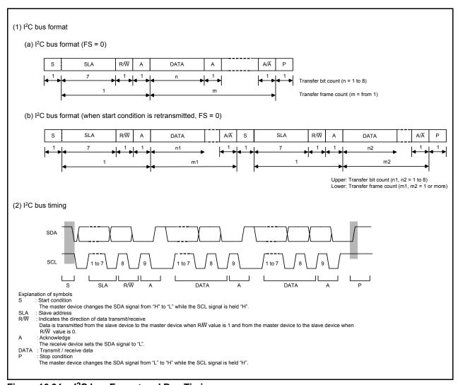
Figure 16.34 I<sup>2</sup>C bus Format and Bus Timing
