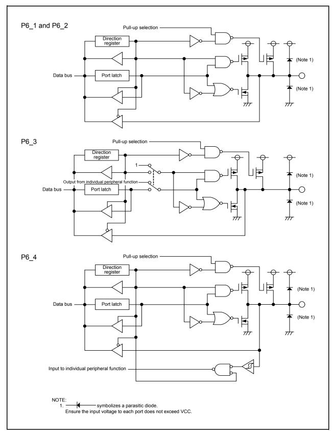
Configuration of Programmable I/O Ports (8) Figure 7.8
