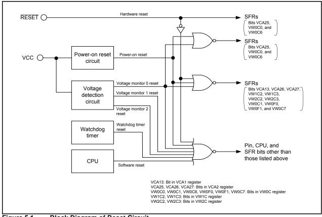
Figure 5.1 Block Diagram of Reset Circuit
