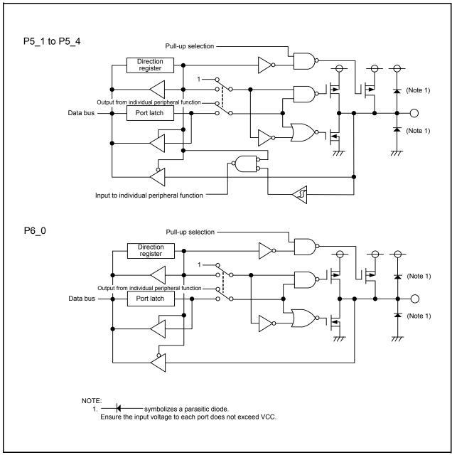
Configuration of Programmable I/O Ports (7) Figure 7.7
