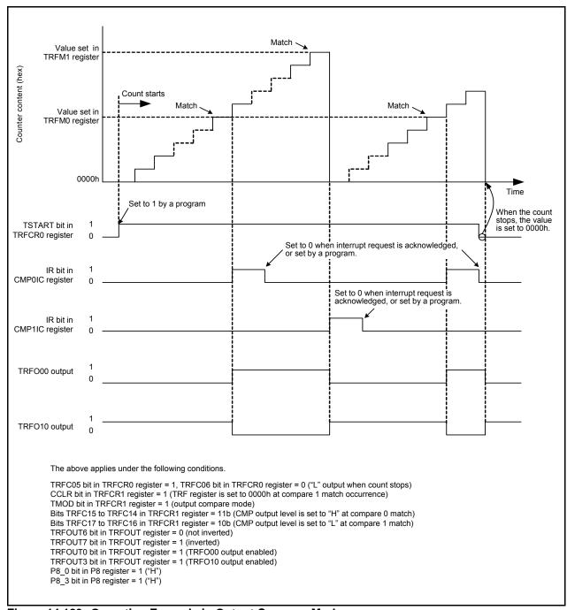
Figure 14.183 Operating Example in Output Compare Mode
