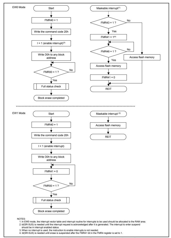
Figure 20.15 Block Erase Command (When Erase-Suspend Function Enabled)
