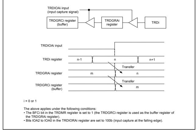
Figure 14.64 Buffer Operation in Input Capture Function
