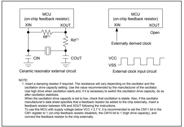
Figure 10.11 Examples of XIN Clock Connection Circuit
