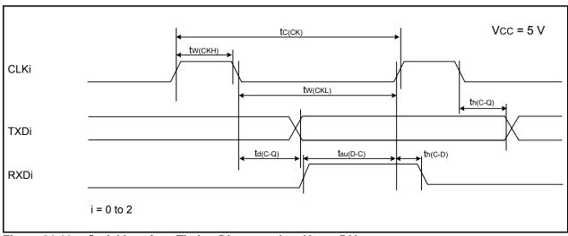
**Figure 21.11** Serial Interface Timing Diagram when Vcc = 5 V
