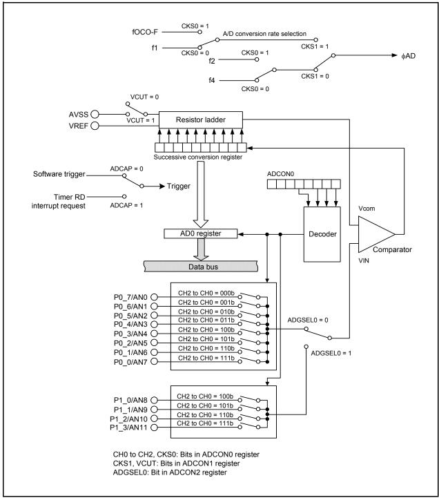
Figure 18.1 Block Diagram of A/D Converter
