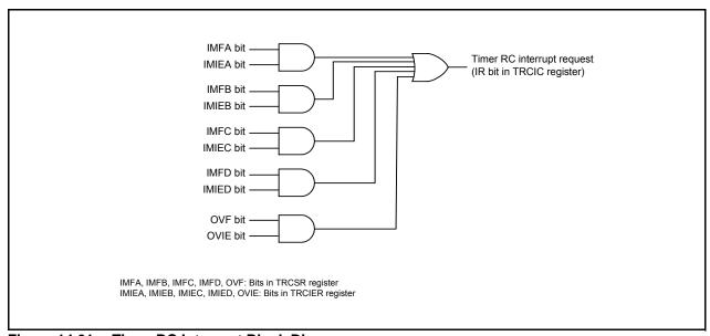
Figure 14.61 Timer RC Interrupt Block Diagram
