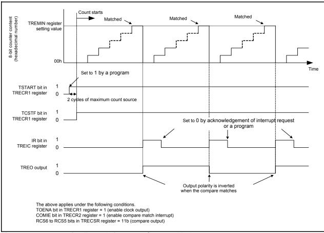
Figure 14.172 Operating Example in Output Compare Mode
