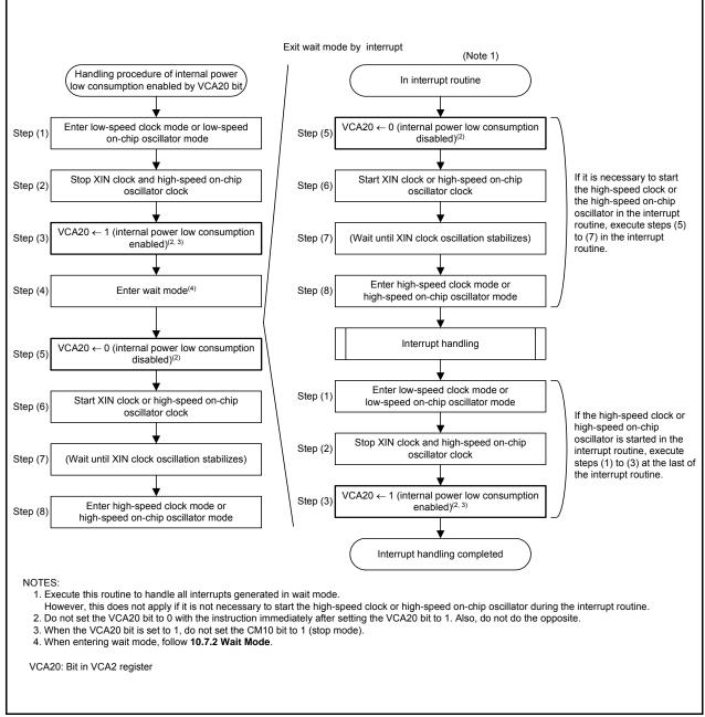
Procedure for Enabling Reduced Internal Power Consumption Using VCA20 bit **Figure 10.14**
