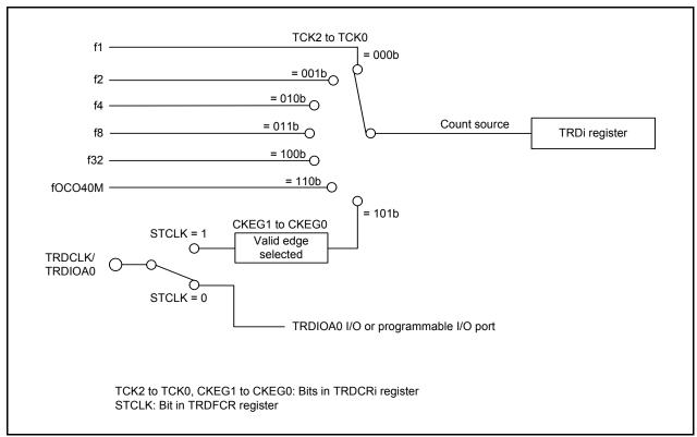
Figure 14.63 Block Diagram of Count Source
