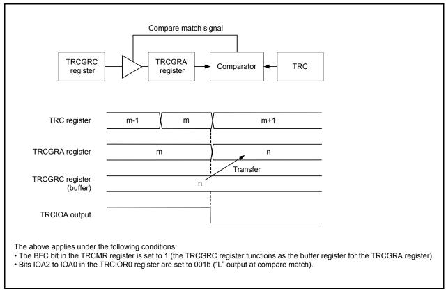
Figure 14.40 Buffer Operation for Output Compare Function
