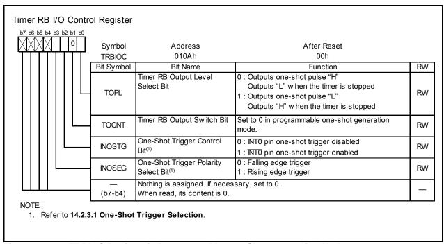
**Figure 14.20** TRBIOC Register in Programmable One-Shot Generation Mode
