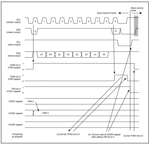
Figure 16.40 Operating Timing in Slave Transmit Mode (I<sup>2</sup>C bus Interface Mode) (2)
