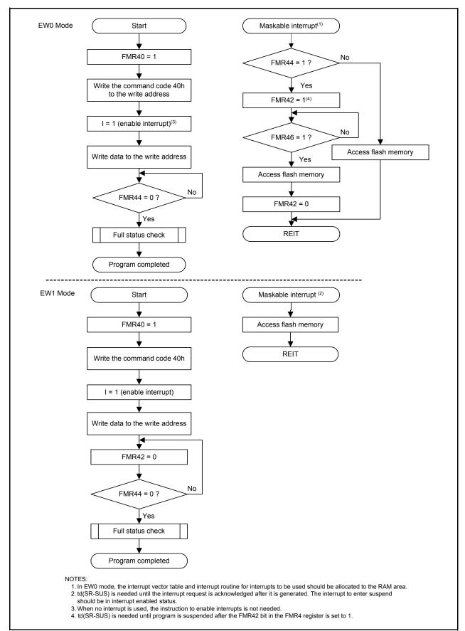
Figure 20.13 Program Command (When Suspend Function Enabled)
