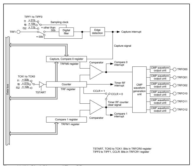
Figure 14.174 Block Diagram of Timer RF
