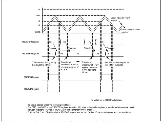
Figure 22.6 Operation when Value in Buffer Register ≥ Value in TRDGRA0 Register in Complementary PWM Mode
