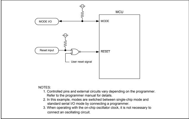
Figure 20.19 Pin Processing in Standard Serial I/O Mode 3
