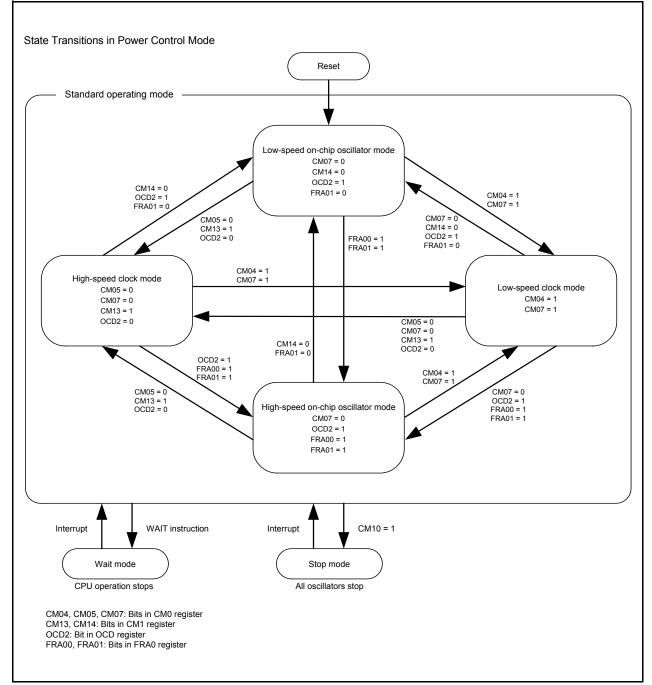
Figure 10.16 shows the State Transitions in Power Control Mode.
