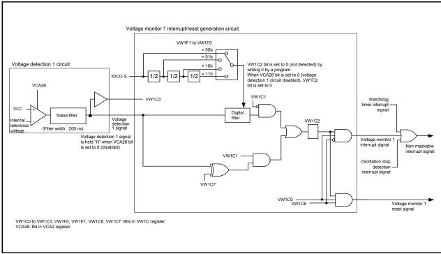
Block Diagram of Voltage Monitor 1 Interrupt/Reset Generation Circuit Figure 6.3
