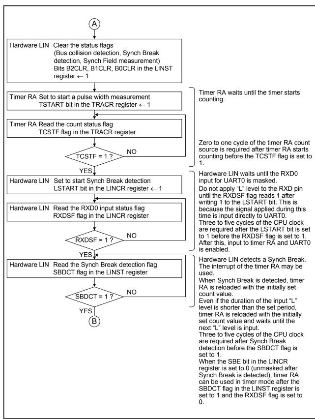
Figure 17.9 **Example of Header Field Reception Flowchart (2)**
