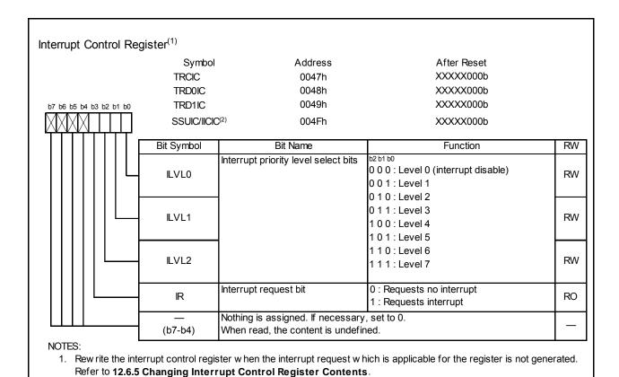
Figure 12.4 Registers TRCIC, TRD0IC, TRD1IC, SSUIC, and IICIC
