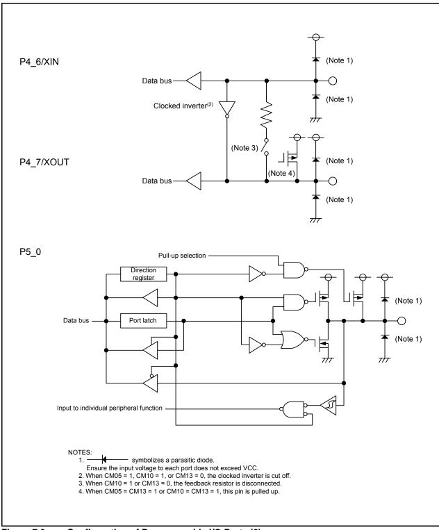
Configuration of Programmable I/O Ports (6) Figure 7.6
