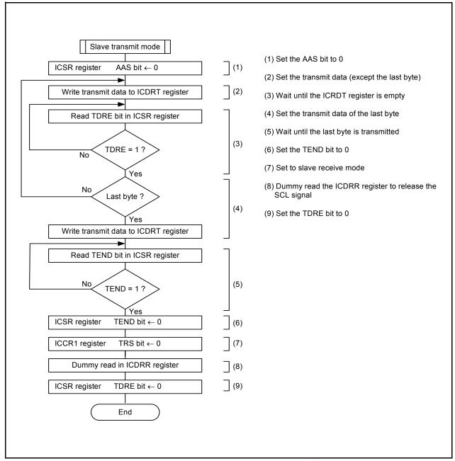
Figure 16.48 Example of Register Setting in Slave Transmit Mode (I<sup>2</sup>C bus Interface Mode)
