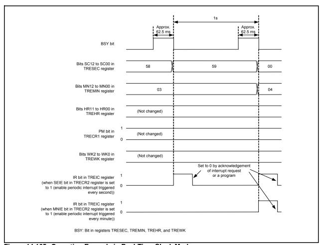
Figure 14.165 Operating Example in Real-Time Clock Mode
