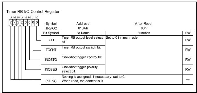
Figure 14.16 TRBIOC Register in Timer Mode
