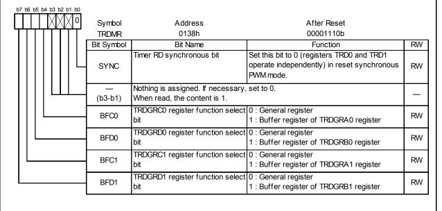
Figure 14.116 Registers TRDSTR and TRDMR in Reset Synchronous PWM Mode
