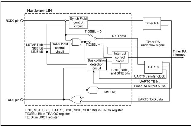
Figure 17.1 **Block Diagram of Hardware LIN**
