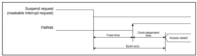
Figure 21.2 Time delay until Suspend
