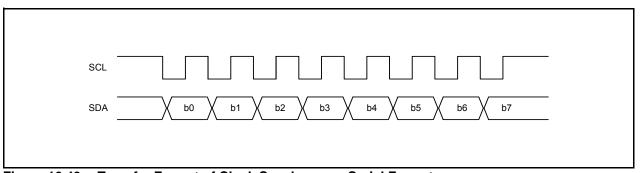
**Figure 16.43 Transfer Format of Clock Synchronous Serial Format**
