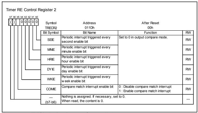
Figure 14.170 TRECR2 Register in Output Compare Mode
