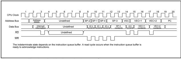
Figure 12.6 Time Required for Executing Interrupt Sequence
