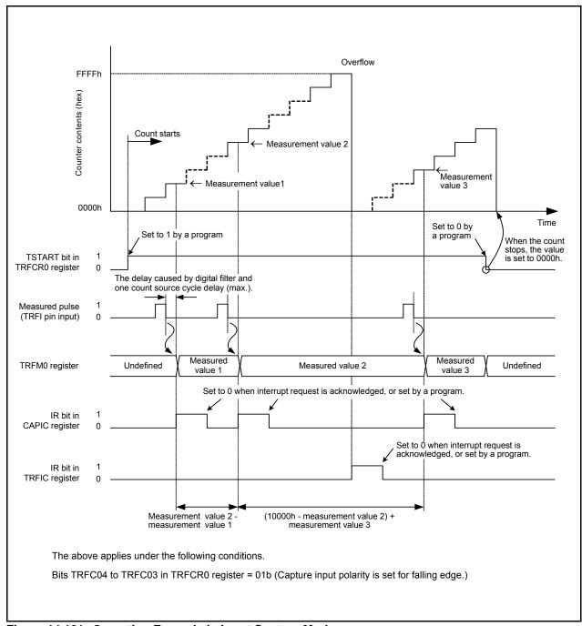
Figure 14.181 Operating Example in Input Capture Mode
