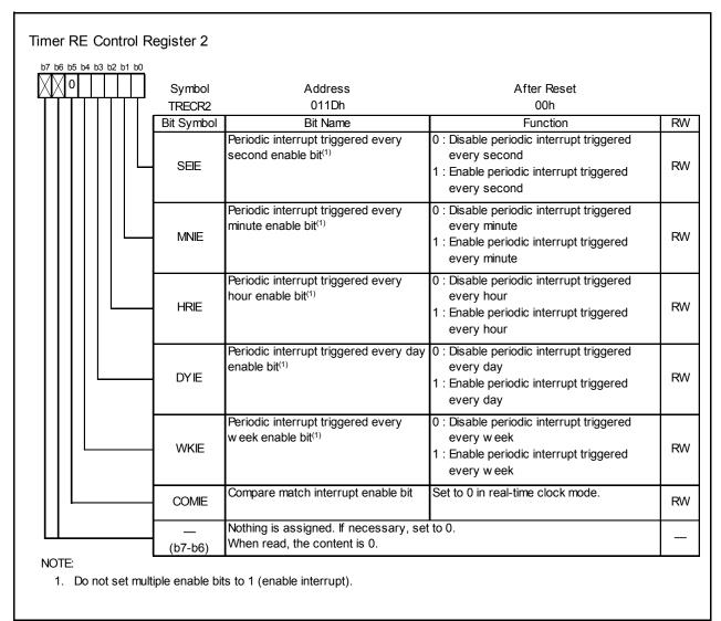
Figure 14.163 TRECR2 Register in Real-Time Clock Mode
