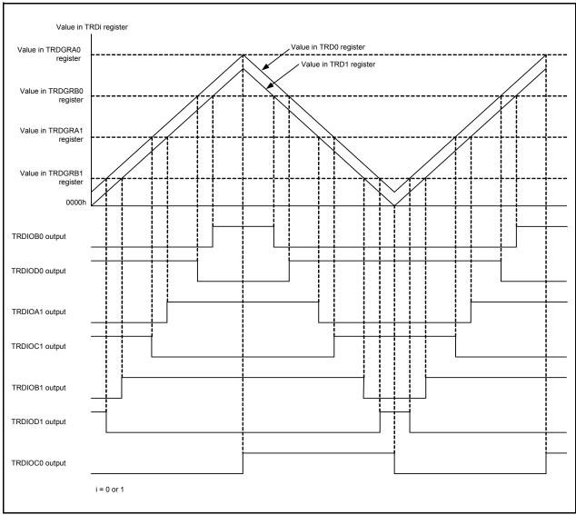
Figure 14.136 Output Model of Complementary PWM Mode
