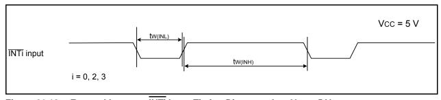
Figure 21.12 External Interrupt INTi Input Timing Diagram when Vcc = 5 V
