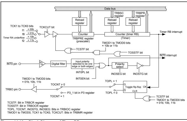
Figure 14.12 Block Diagram of Timer RB
