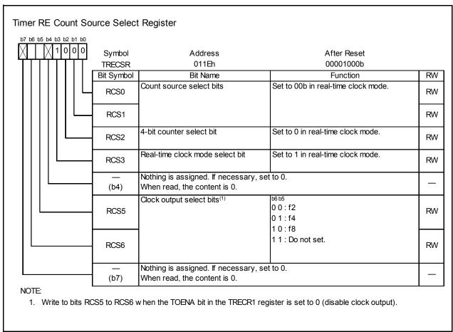
Figure 14.164 TRECSR Register in Real-Time Clock Mode
