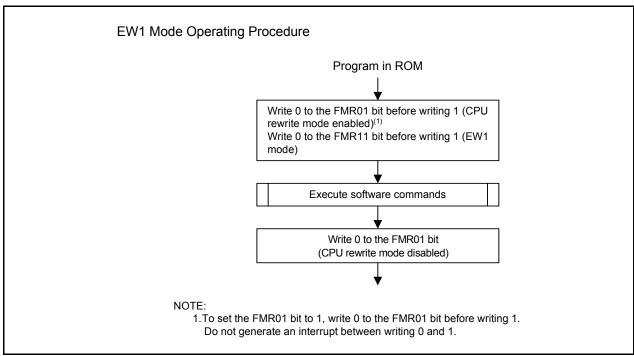
Figure 20.10 How to Set and Exit EW1 Mode
