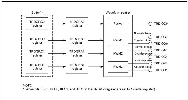
Figure 14.114 Block Diagram of Reset Synchronous PWM Mode
