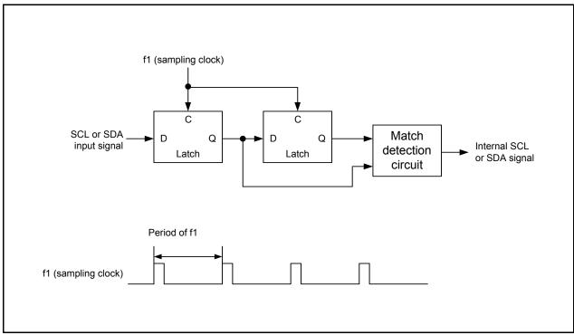
**Figure 16.50 Block Diagram of Noise Canceller**
