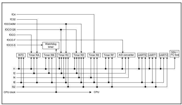
Figure 10.2 **Peripheral Function Clock**
