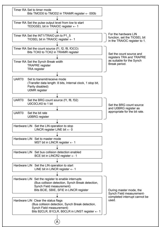
Figure 17.5 Example of Header Field Transmission Flowchart (1)
