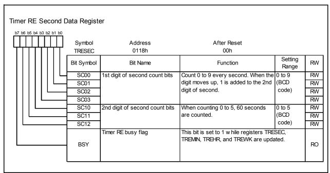
Figure 14.157 TRESEC Register in Real-Time Clock Mode
