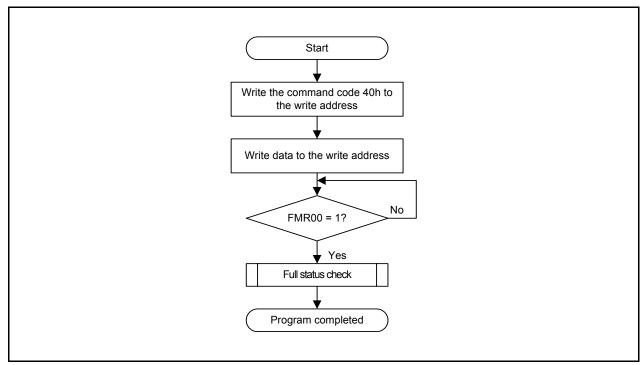
Figure 20.12 Program Command (When Suspend Function Disabled)
