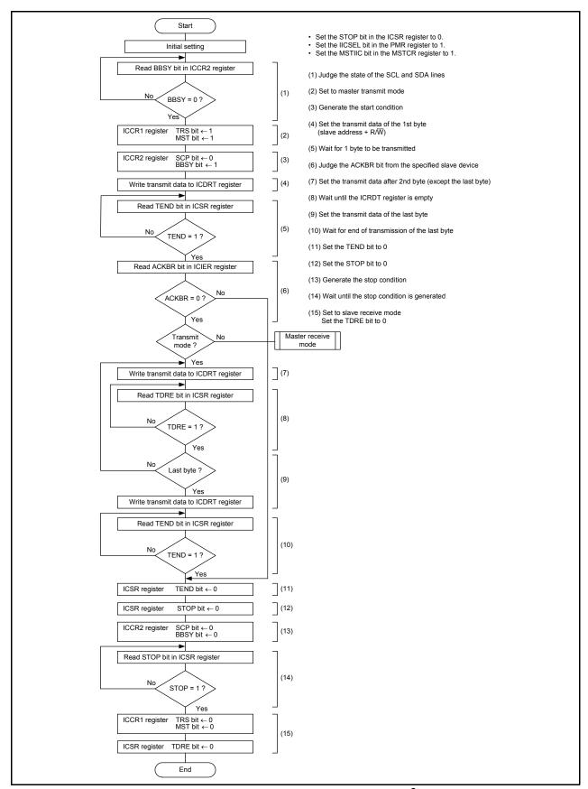
Figure 16.46 Example of Register Setting in Master Transmit Mode (I<sup>2</sup>C bus Interface Mode)
