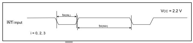
Figure 21.22 External Interrupt INTi Input Timing Diagram when Vcc = 2.2 V
