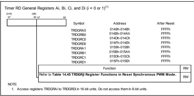
Figure 14.123 Registers TRDGRAi, TRDGRBi, TRDGRCi, and TRDGRDi in Reset Synchronous PWM Mode
