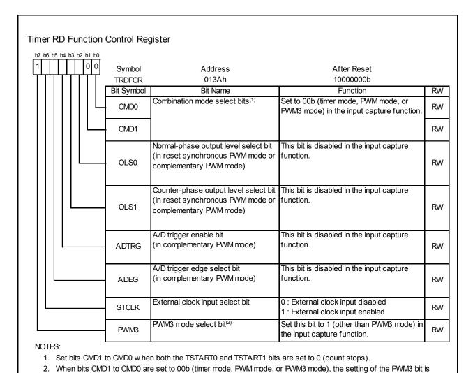
**Figure 14.72 TRDFCR Register in Input Capture Function**
