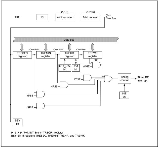
Figure 14.156 Block Diagram of Real-Time Clock Mode
