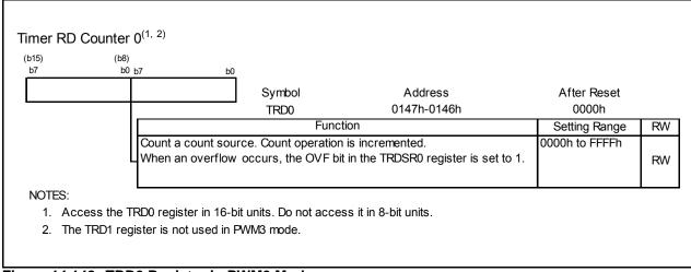
Figure 14.148 TRD0 Register in PWM3 Mode
