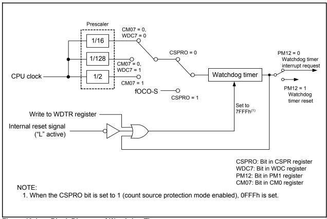
Figure 13.1 Block Diagram of Watchdog Timer
