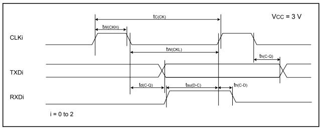
**Figure 21.16** Serial Interface Timing Diagram when Vcc = 3 V
