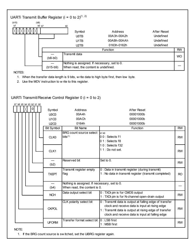
Figure 15.5 Registers U0TB to U2TB and U0C0 to U2C0
