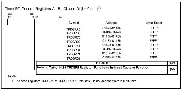
Figure 14.80 Registers TRDGRAi, TRDGRBi, TRDGRCi, and TRDGRDi in Input Capture Function
