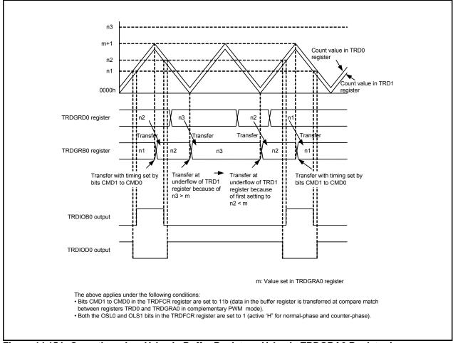
Figure 14.154 Operation when Value in Buffer Register ≥ Value in TRDGRA0 Register in Complementary PWM Mode
