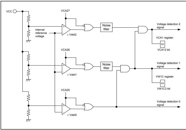
Figure 6.1 Block Diagram of Voltage Detection Circuit
