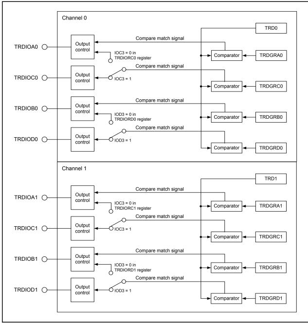
Figure 14.83 Block Diagram of Output Compare Function
