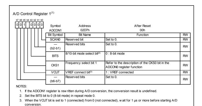
Figure 18.8 ADCON1 Register in Repeat Mode 0
