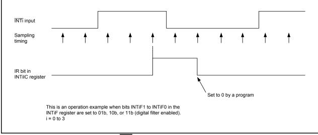
Figure 12.17 Operating Example of INTi Input Filter
