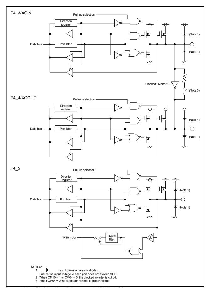
Configuration of Programmable I/O Ports (5) Figure 7.5
