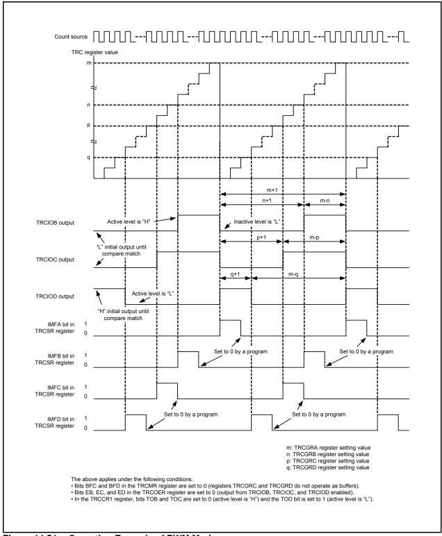
Figure 14.54 Operating Example of PWM Mode
