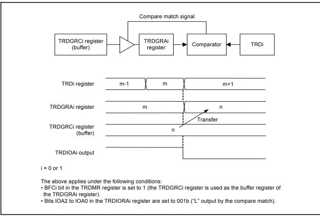
Figure 14.65 Buffer Operation in Output Compare Function
