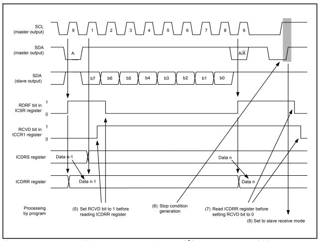
Operating Timing in Master Receive Mode (I<sup>2</sup>C bus Interface Mode) (2) **Figure 16.38**
