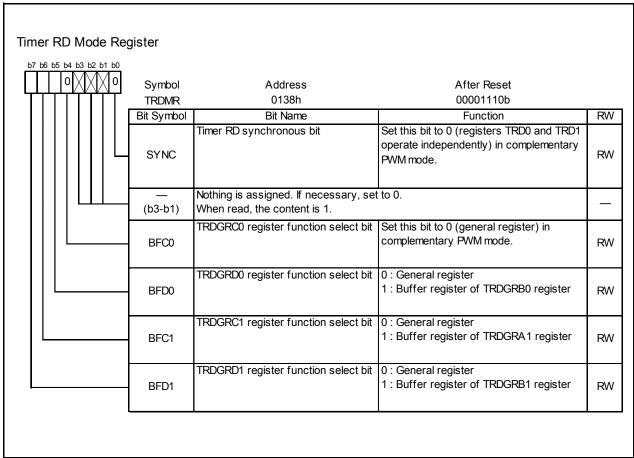
Figure 14.128 TRDMR Register in Complementary PWM Mode
