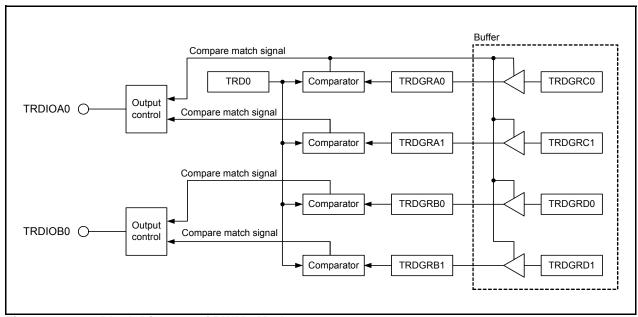
Figure 14.138 Block Diagram of PWM3 Mode
