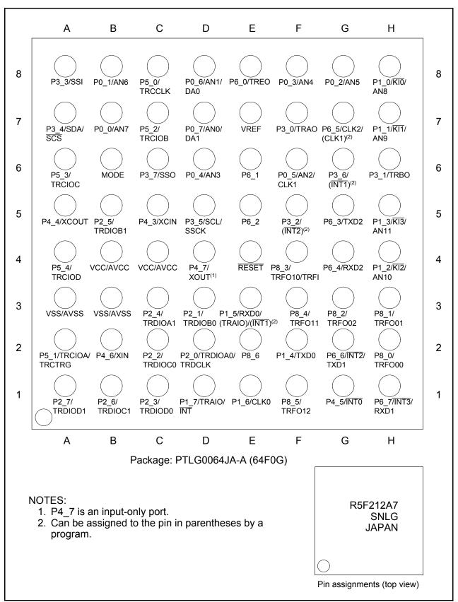
64-pin FLGA Package Pin Assignment (Top Perspective View) Figure 1.5
