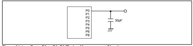
Ports P0 to P6, P8 Timing Measurement Circuit Figure 21.1
