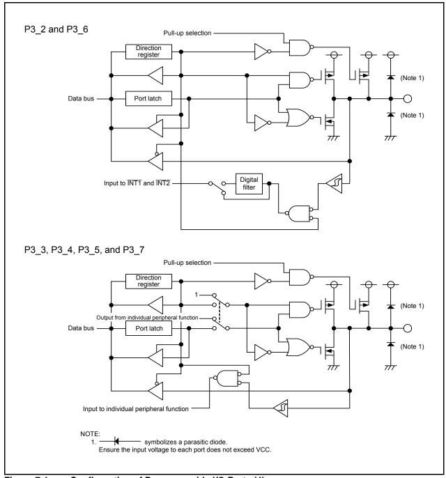
Figure 7.4 Configuration of Programmable I/O Ports (4)
