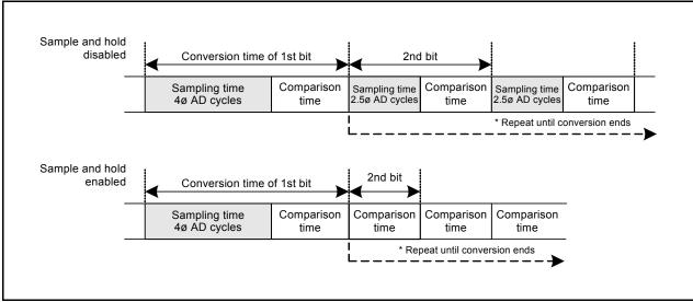
Figure 18.9 Timing Diagram of A/D Conversion
