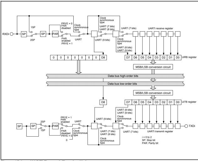
Figure 15.2 UARTi Transmit/Receive Unit
