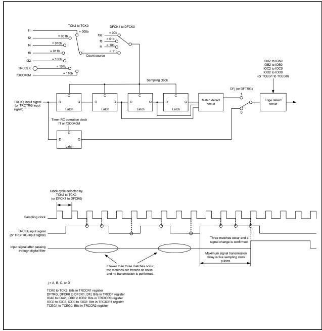
Figure 14.41 Block Diagram of Digital Filter
