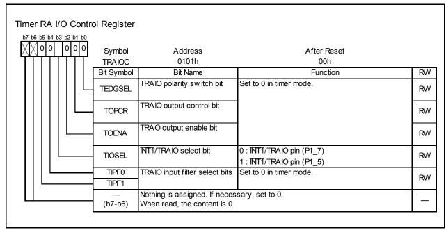
Figure 14.4 TRAIOC Register in Timer Mode
