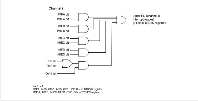
Figure 12.21 Block Diagram of Timer RD Interrupt
