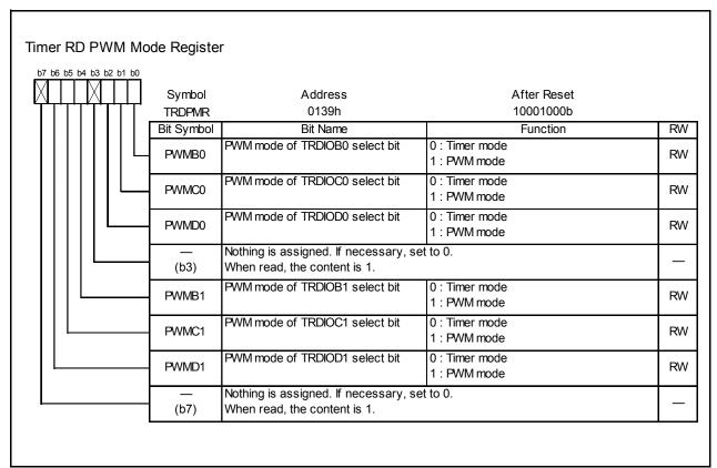
Figure 14.103 TRDPMR Register in PWM Mode
