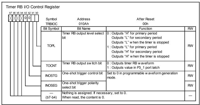
Figure 14.18 TRBIOC Register in Programmable Waveform Generation Mode
