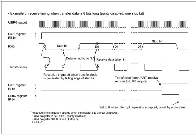
Figure 15.13 Receive Timing Example in UART Mode
