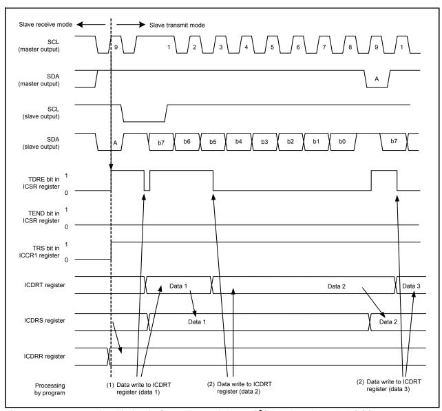
Figure 16.39 Operating Timing in Slave Transmit Mode (I<sup>2</sup>C bus Interface Mode) (1)
