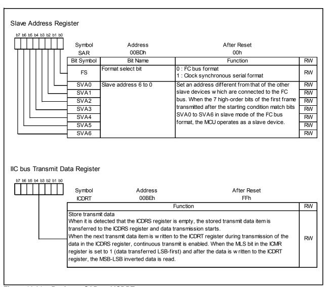
Figure 16.31 Registers SAR and ICDRT
