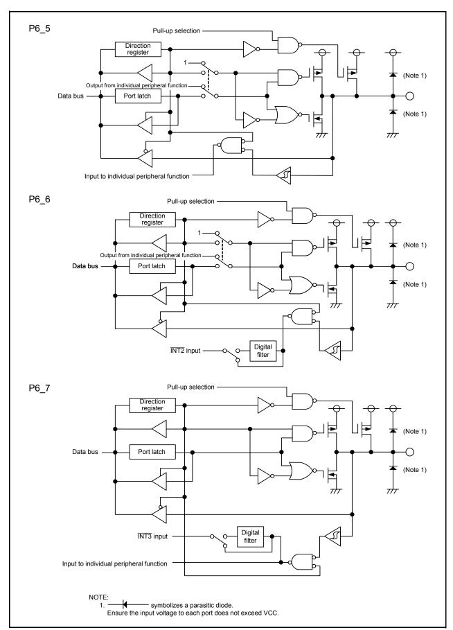
Figure 7.9 Configuration of Programmable I/O Ports (9)
