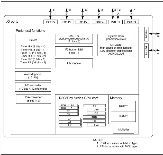
Figure 1.3 Block Diagram
