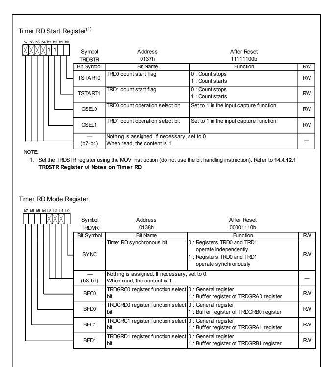
Figure 14.70 Registers TRDSTR and TRDMR in Input Capture Function
