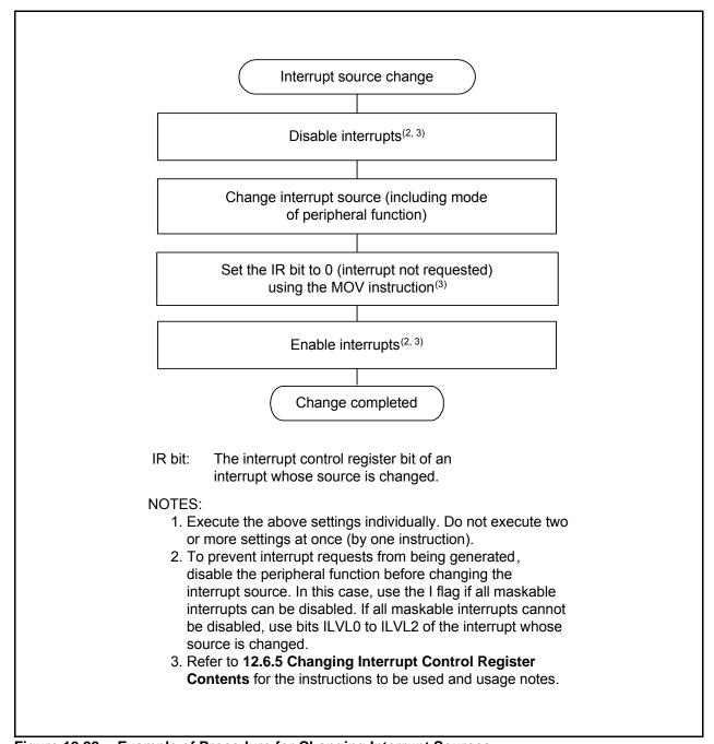
Figure 12.22 Example of Procedure for Changing Interrupt Sources
