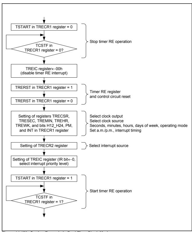
Figure 14.173 Setting Example in Real-Time Clock Mode
