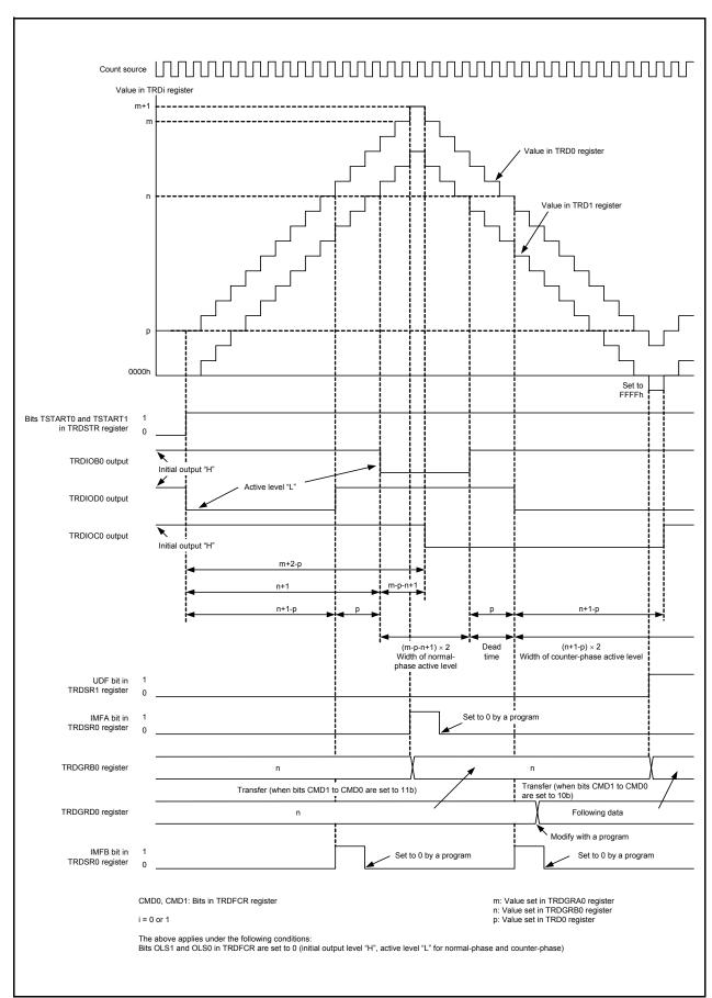
Figure 14.137 Operating Example of Complementary PWM Mode
