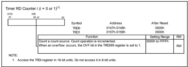
Figure 14.95 Registers TRD0 to TRD1 in Output Compare Function
