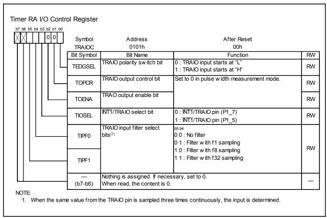
Figure 14.8 TRAIOC Register in Pulse Width Measurement Mode
