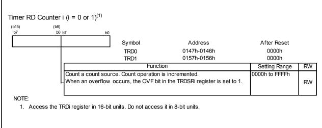
Figure 14.110 Registers TRD0 to TRD1 in PWM Mode
