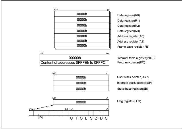
Figure 5.2 **CPU Register Status after Reset**
