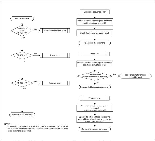
Full Status Check and Handling Procedure for Individual Errors
