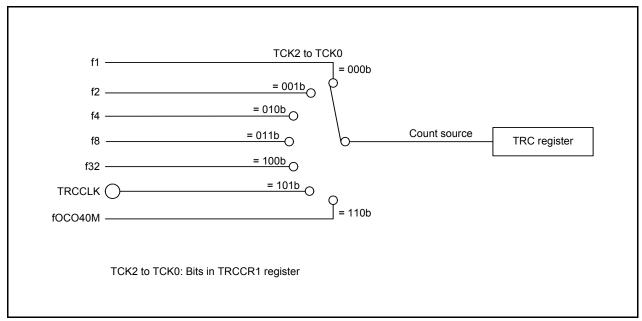
Figure 14.38 Count Source Block Diagram
