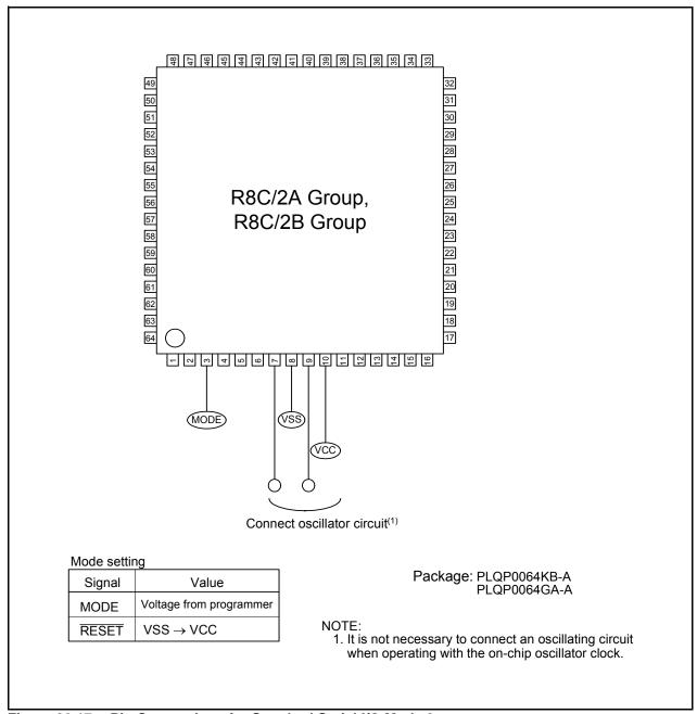
Figure 20.17 Pin Connections for Standard Serial I/O Mode 3
