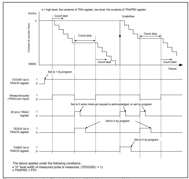
Figure 14.9 Operating Example of Pulse Width Measurement Mode
