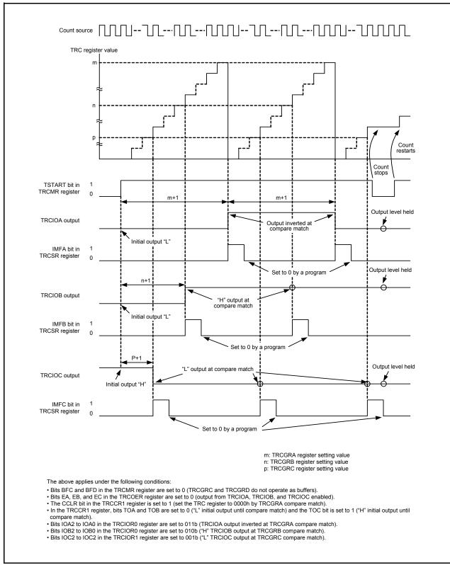
**Figure 14.51 Operating Example of Output Compare Function**
