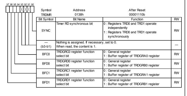
Figure 14.102 Registers TRDSTR and TRDMR in PWM Mode
