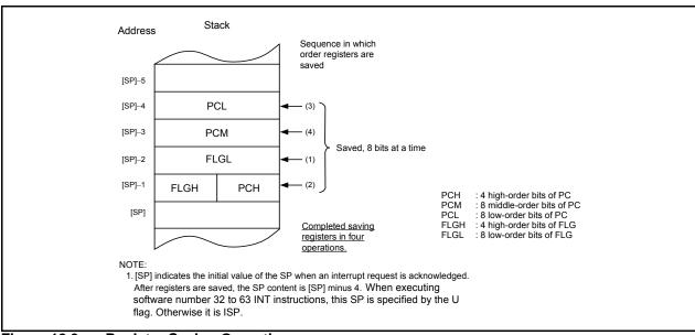
Figure 12.9 Register Saving Operation
