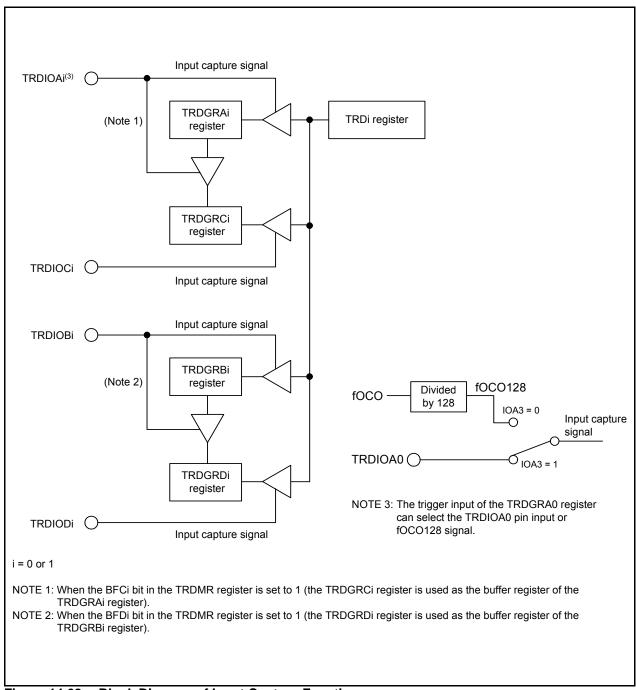
Figure 14.68 **Block Diagram of Input Capture Function**
