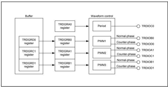
Figure 14.125 Block Diagram of Complementary PWM Mode
