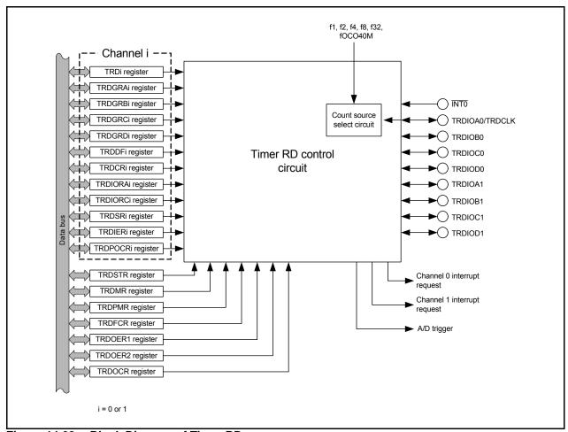
Figure 14.62 Block Diagram of Timer RD
