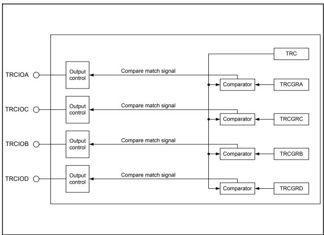
**Figure 14.47 Block Diagram of Output Compare Function**
