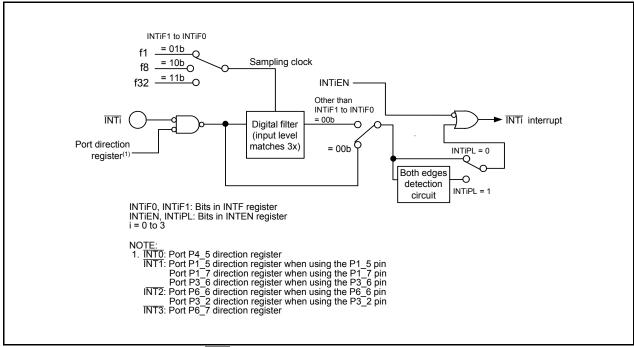
Figure 12.16 Configuration of INTi Input Filter
