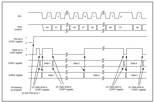
Operating Timing in Transmit Mode (Clock Synchronous Serial Mode) **Figure 16.44**
