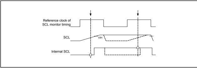
Figure 16.51 Timing of Bit Synchronization Circuit
