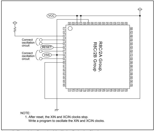
Appendix Figure 3.1 Example of Oscillation Evaluation Circuit
