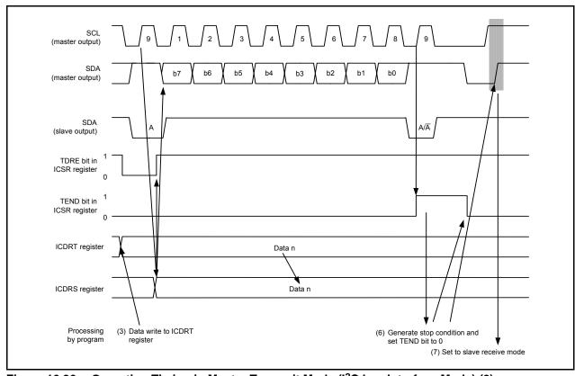
Figure 16.36 Operating Timing in Master Transmit Mode (I<sup>2</sup>C bus Interface Mode) (2)
