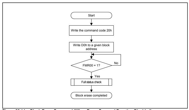
Figure 20.14 Block Erase Command (When Erase-Suspend Function Disabled)
