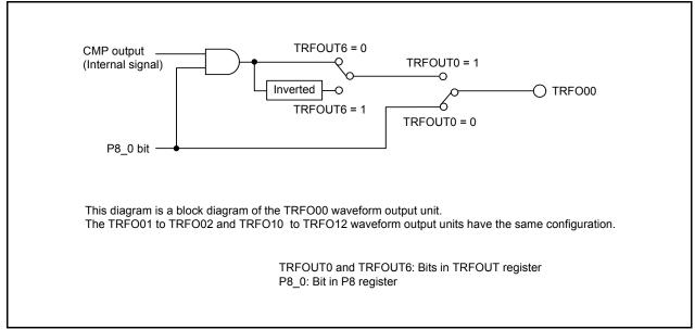
Figure 14.176 Block Diagram of CMP Waveform Output Unit
