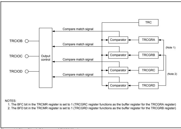
**Figure 14.52 Block Diagram of PWM Mode**
