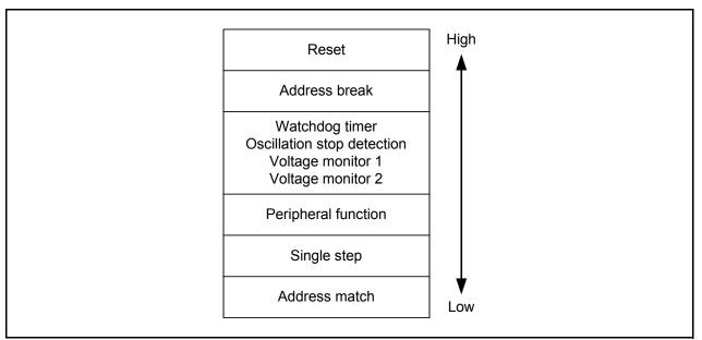
Figure 12.10 Priority Levels of Hardware Interrupts
