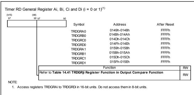
Figure 14.96 Registers TRDGRAi, TRDGRBi, TRDGRCi, and TRDGRDi in Output Compare Function
