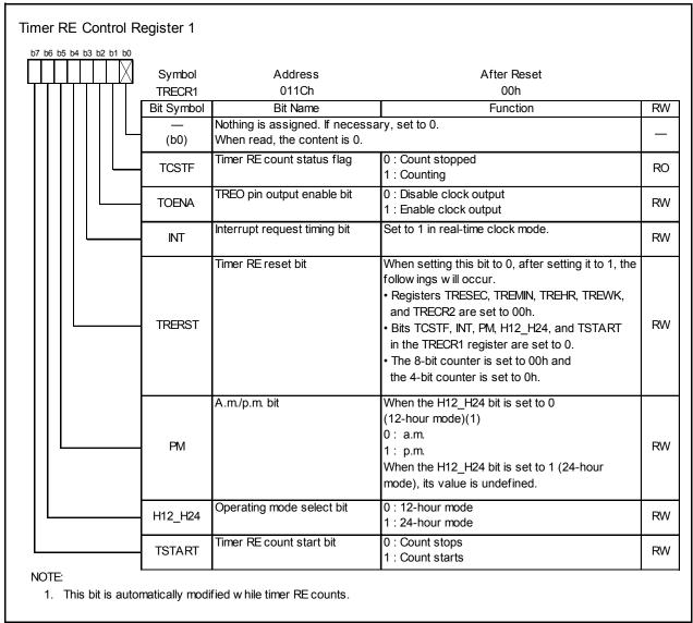
Figure 14.161 TRECR1 Register in Real-Time Clock Mode
