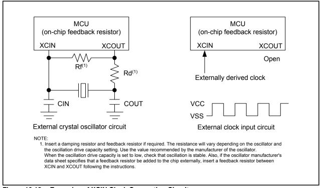
Figure 10.12 Examples of XCIN Clock Connection Circuits
