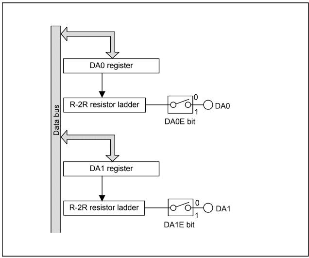
Figure 19.1 **Block Diagram of D/A Converter**
