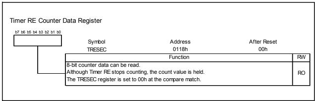
Figure 14.167 TRESEC Register in Output Compare Mode
