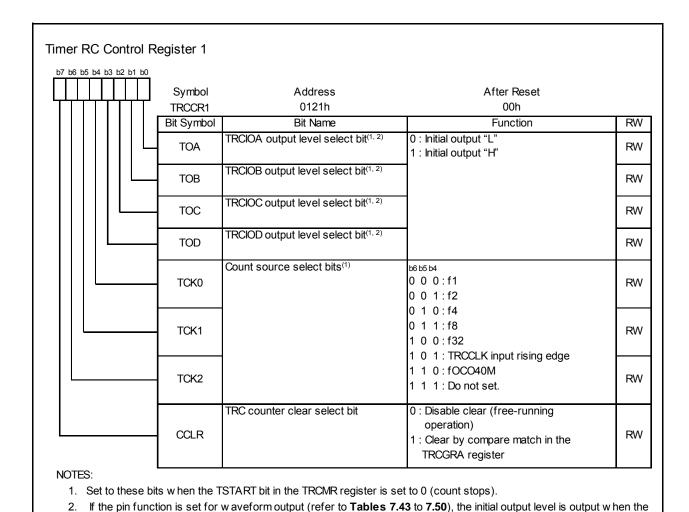
**Figure 14.50 TRCCR1 Register for Output Compare Function**
