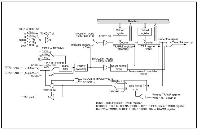
Figure 14.1 Block Diagram of Timer RA
