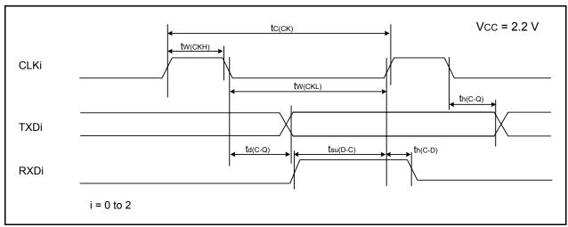
Figure 21.21 Serial Interface Timing Diagram when Vcc = 2.2 V
