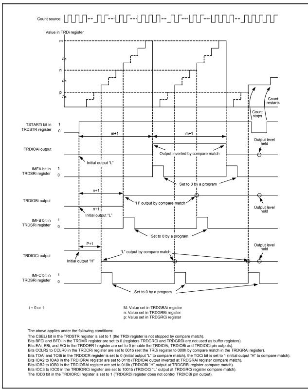
Figure 14.97 Operating Example of Output Compare Function
