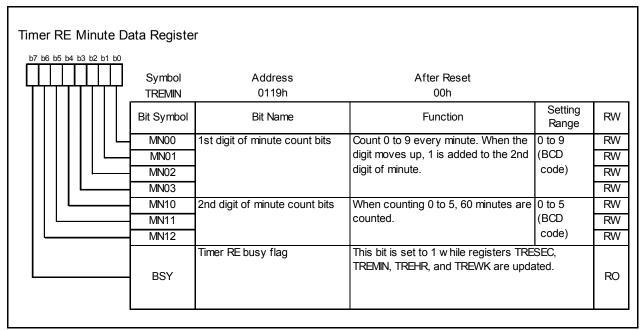
Figure 14.158 TREMIN Register in Real-Time Clock Mode
