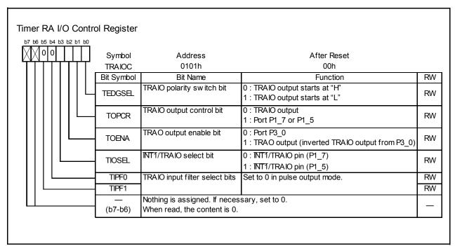
Figure 14.6 **TRAIOC Register in Pulse Output Mode**
