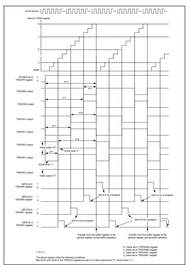
Figure 14.124 Operating Example of Reset Synchronous PWM Mode
