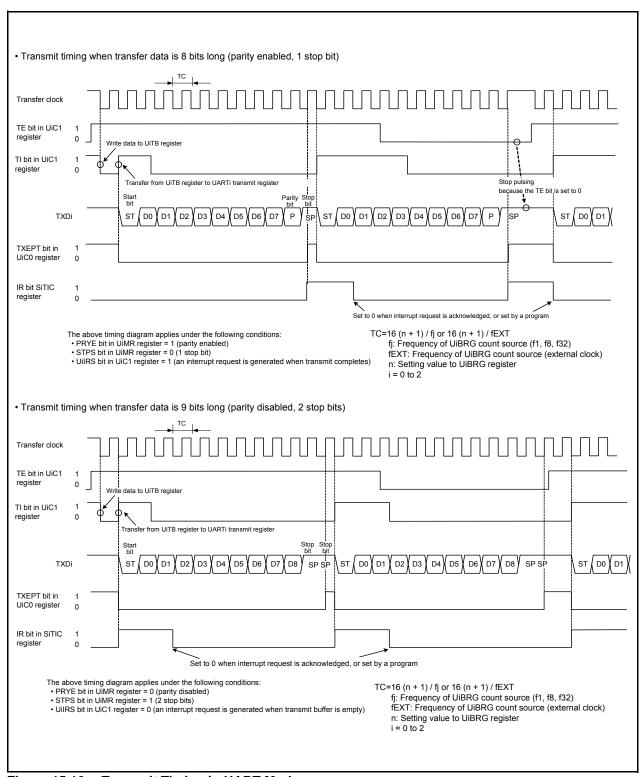
Figure 15.12 Transmit Timing in UART Mode
