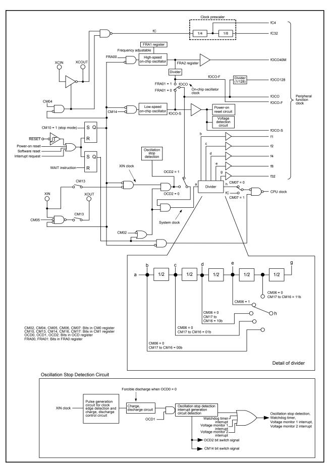
Figure 10.1 **Clock Generation Circuit**
