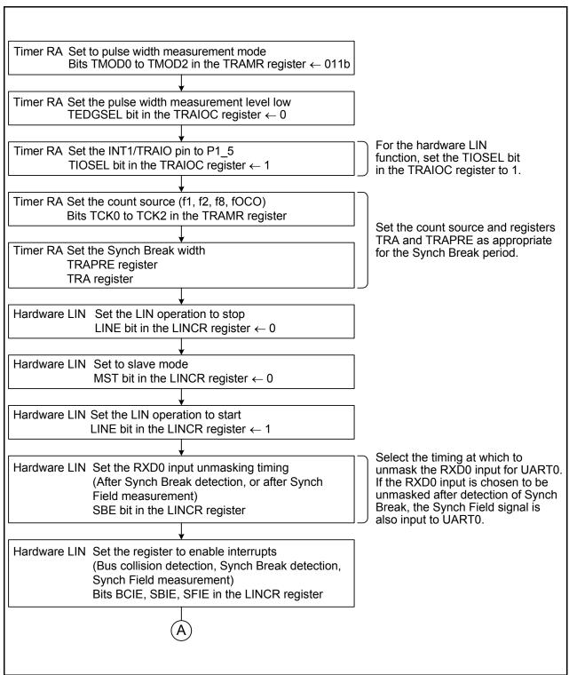
Figure 17.8 Example of Header Field Reception Flowchart (1)
