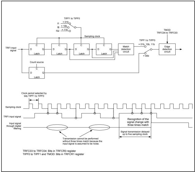
Figure 14.182 Block Diagram of Digital Filter
