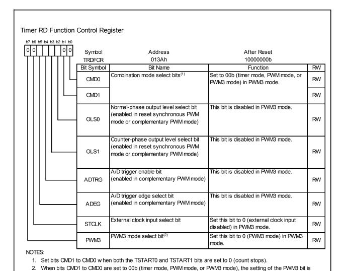
Figure 14.142 TRDFCR Register in PWM3 Mode
