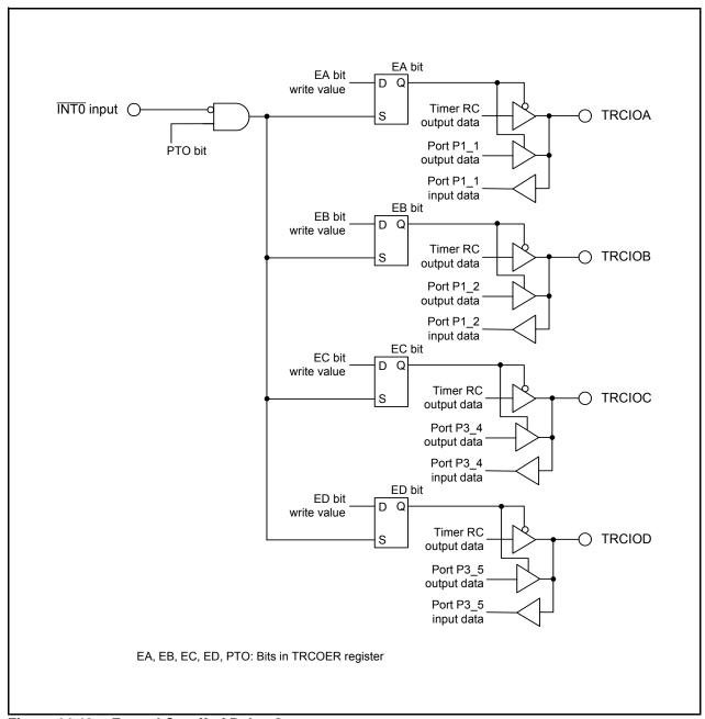
Figure 14.42 Forced Cutoff of Pulse Output
