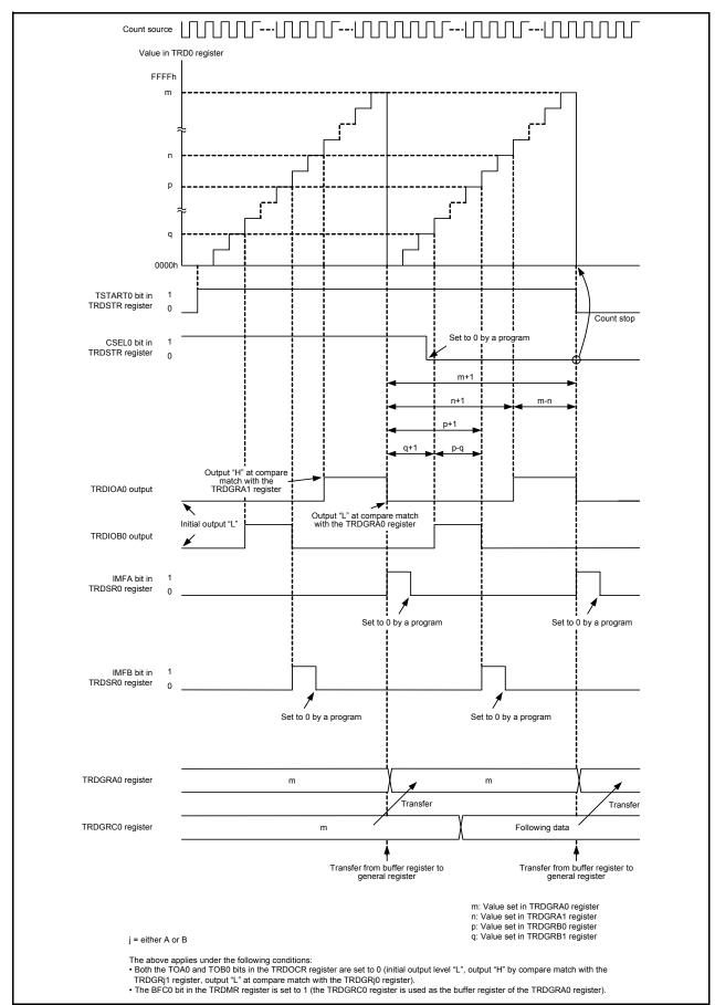
Figure 14.150 Operating Example of PWM3 Mode
