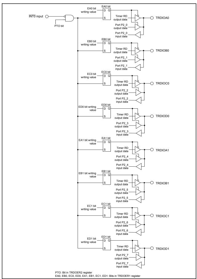
Figure 14.67 Pulse Output Forced Cutoff
