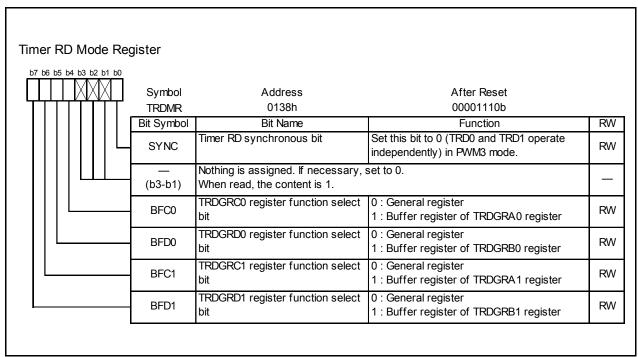
Figure 14.141 TRDMR Register in PWM3 Mode
