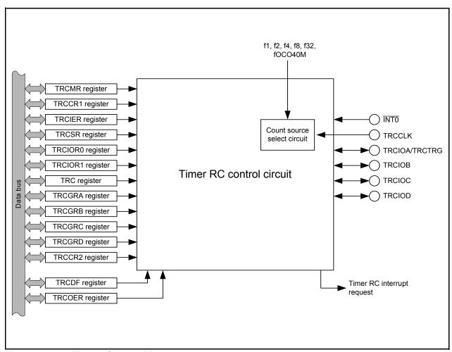
Figure 14.26 Timer RC Block Diagram
