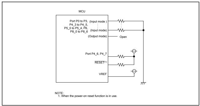
Figure 7.17 Unassigned Pin Handling
