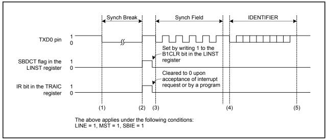
Figure 17.4 Typical Operation when Sending a Header Field
