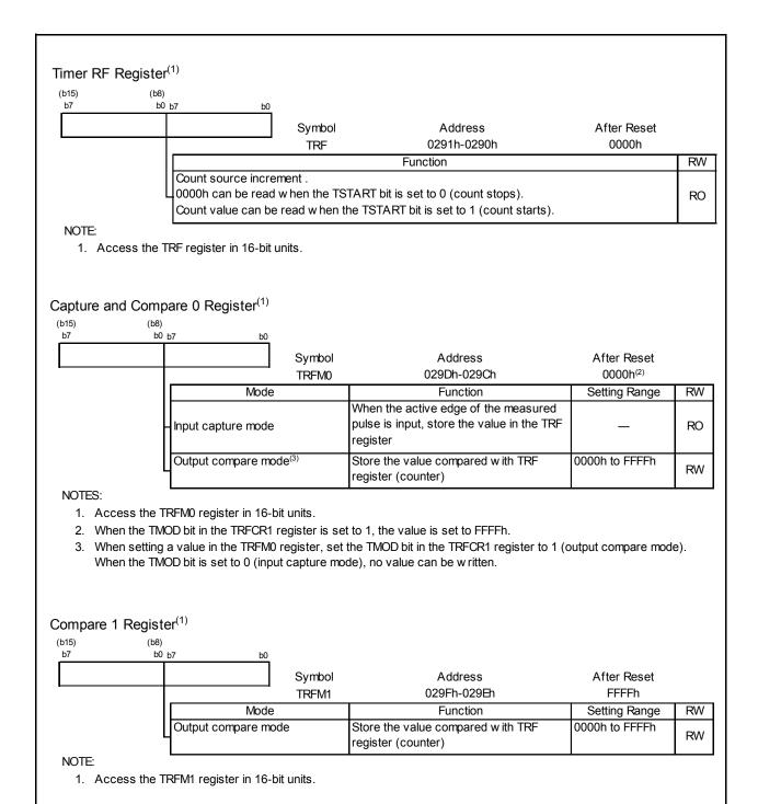
Figure 14.177 Registers TRF, TRFM0, and TRFM1
