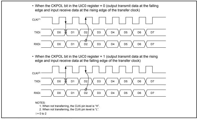
Figure 15.10 Transfer Clock Polarity
