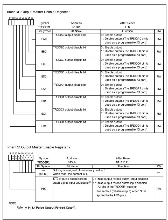
Figure 14.105 Registers TRDOER1 to TRDOER2 in PWM Mode
