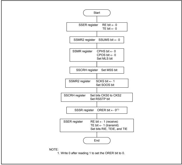
Figure 16.13 Initialization in Clock Synchronous Communication Mode
