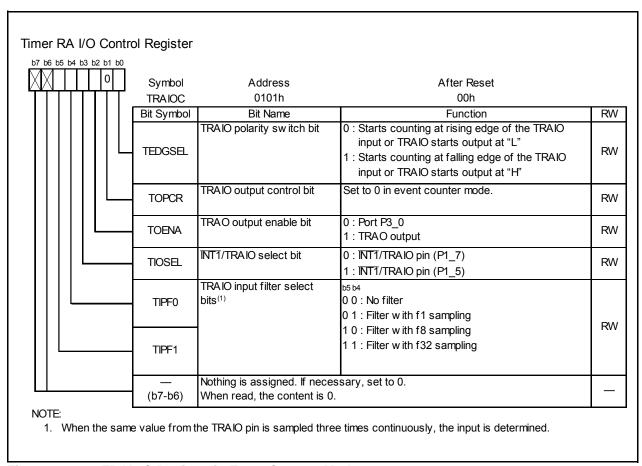
Figure 14.7 **TRAIOC Register in Event Counter Mode**
