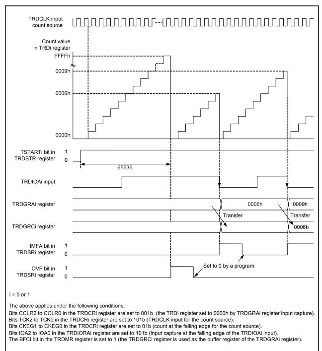
Figure 14.81 Operating Example of Input Capture Function
