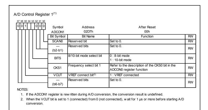
Figure 18.6 **ADCON1 Register in One-Shot Mode**
