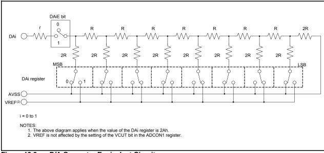
Figure 19.3 D/A Converter Equivalent Circuit
