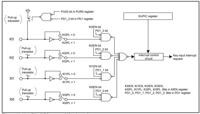
Figure 12.18 Block Diagram of Key Input Interrupt
