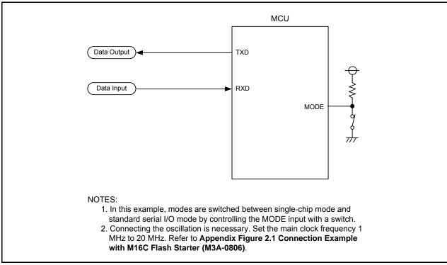
Figure 20.18 Pin Processing in Standard Serial I/O Mode 2
