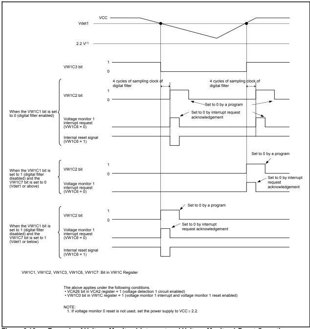
Example of Voltage Monitor 1 Interrupt and Voltage Monitor 1 Reset Operation Figure 6.10
