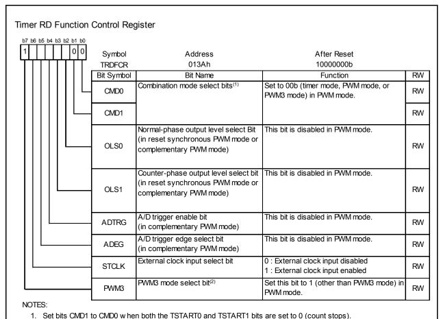
Figure 14.104 TRDFCR Register in PWM Mode
