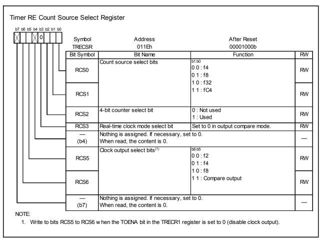
Figure 14.171 TRECSR Register in Output Compare Mode
