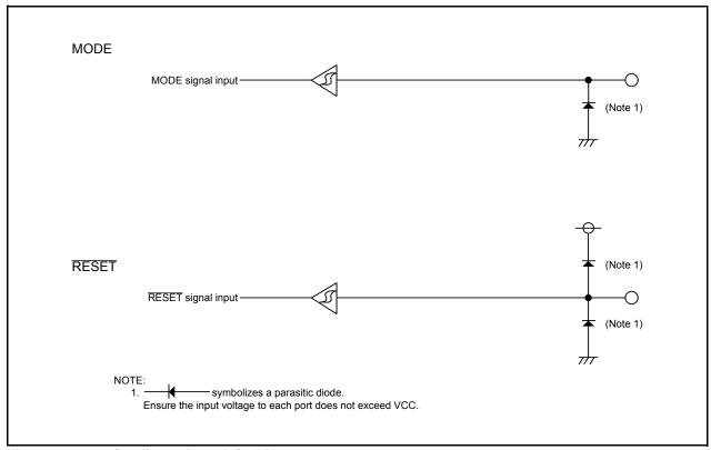
Figure 7.11 Configuration of I/O Pins
