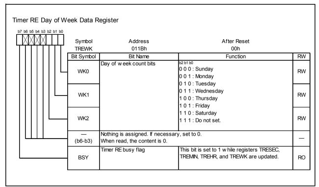
Figure 14.160 TREWK Register in Real-Time Clock Mode
