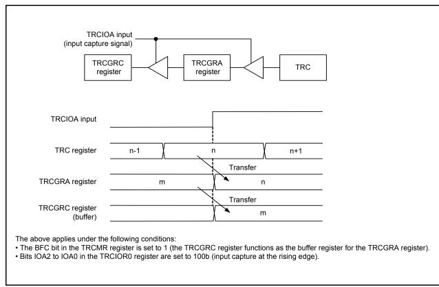
Figure 14.39 Buffer Operation for Input Capture Function
