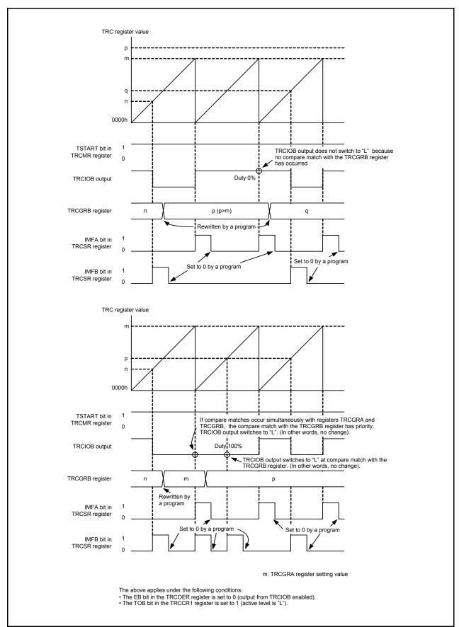
Figure 14.55 Operating Example of PWM Mode (Duty 0% and Duty 100%)
