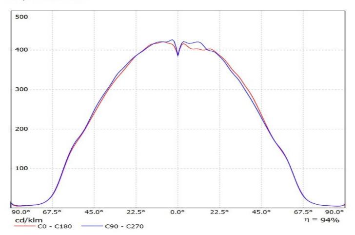
Luminaire: Ledil Oy CS16324\_STRADELLA-IP-28-HB-W\_(J\_Series\_3030\_-\_JK3030\_3V)\_SIMULATED Lamps: 1 x Cree JK3030 3V
