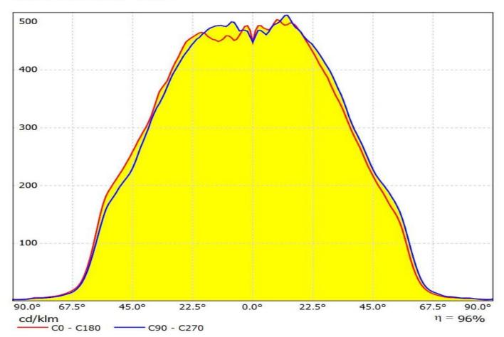
Luminaire: Ledil Oy CS16324\_STRADELLA-IP-28-HB-W\_(Oslon SSL 150)\_SIMULATED Lamps: 1 x Osram Oslon SSL 150 (GW\_CSHPM1pm)
