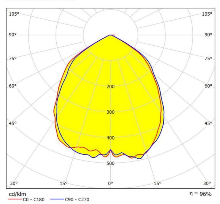
Luminaire: Ledil Oy CS16324\_STRADELLA-IP-28-HB-W\_(Oslon SSL 150)\_SIMULATED Lamps: 1 x Osram Oslon SSL 150 (GW\_CSHPM1pm)
