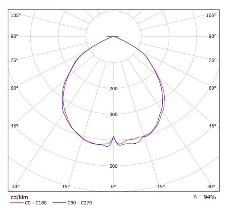
Luminaire: Ledil Oy CS16324\_STRADELLA-IP-28-HB-W\_(J\_Series\_3030\_-\_JK3030\_3V)\_SIMULATED Lamps: 1 x Cree JK3030 3V
