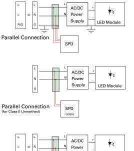
Supply LED Module N/G  $\Sigma^{\Rightarrow}$  LED normally on **Parallel Connection** SPD With LED indicating SPD status LSP10xxxS - ON (green): SPD is online - OFF: SPD needs replacement
