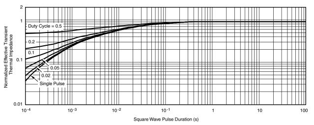
Normalized Thermal Transient Impedance, Junction-to-Case
