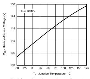
Drain Source Breakdown vs. Junction Temperature
