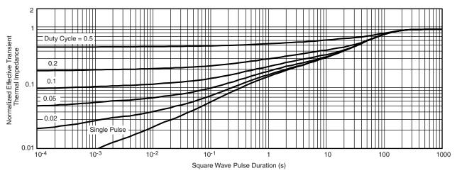
Normalized Thermal Transient Impedance, Junction-to-Ambient
