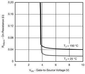
On-Resistance vs. Gate-to-Source Voltage
