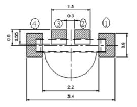
Suggested pad dimension is just for reference only. Please modify the pad dimension based on individual need. Note: Tolerances unless mentioned ±0.1mm. Unit = mm
