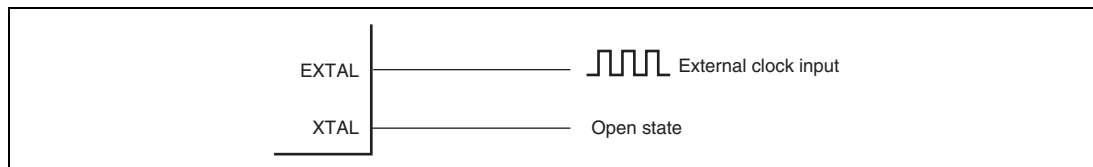
Figure 4.4 Example of External Clock Connection
