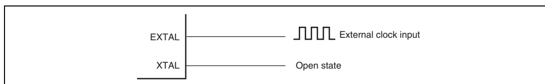
Figure 4.4 Example of External Clock Connection
