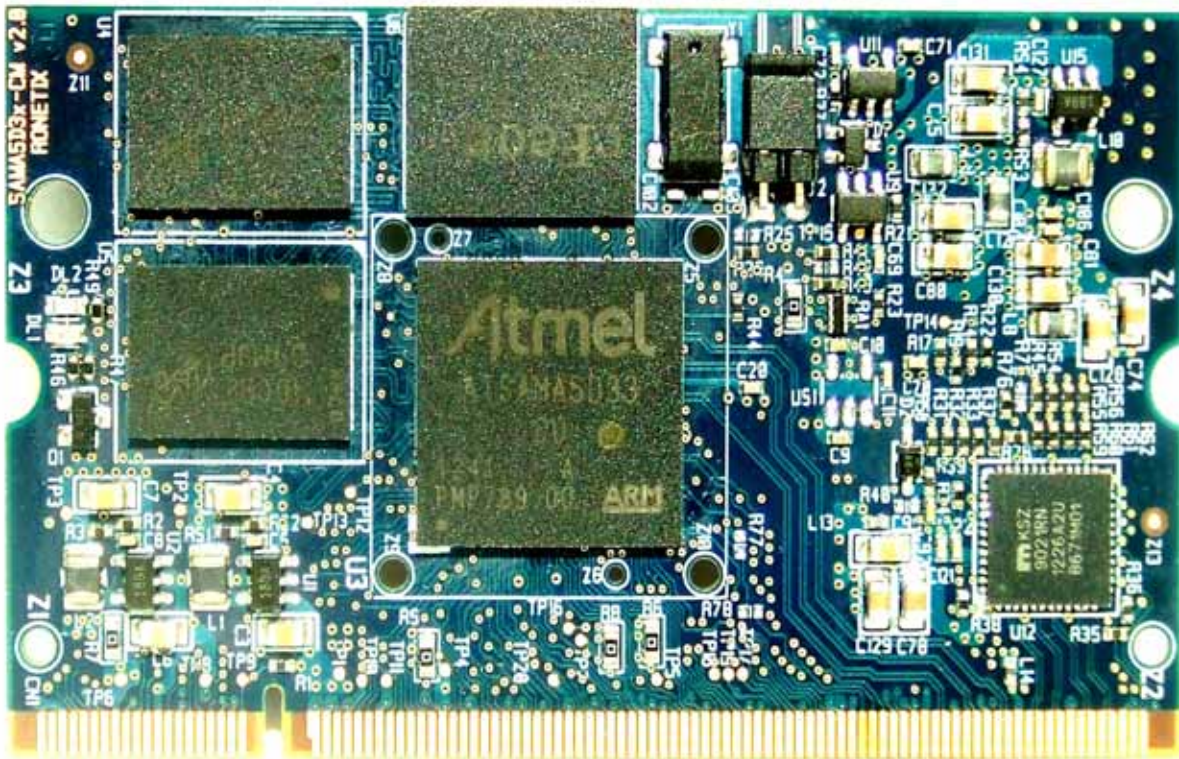
Figure 4-2. CPU Module Board from Ronetix
