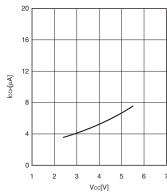
$I_{CCMCR} - V_{CC}$  $T_A = +25^{\circ}C$ ,  $F_{MP} = 4$  MHz (no division) Main CR clock mode
