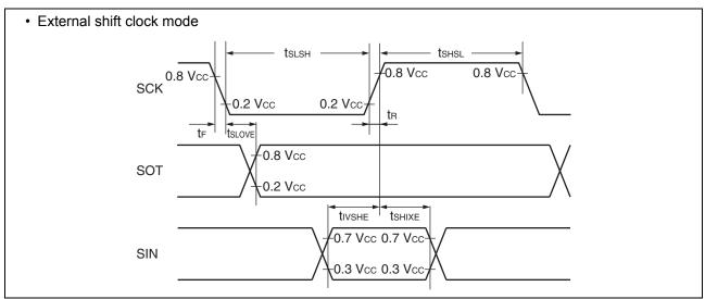
Sampling is executed at the falling edge of the sampling clock\*1, and serial clock delay is disabled\*2. (ESCR register : SCES bit = 1, ECCR register : SCDE bit = 0)
