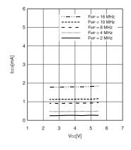
$I_{CCL} - V_{CC}$  $T_A = +25^{\circ}C$ ,  $F_{MPL} = 16$  kHz (divided by 2) Subclock mode with the external clock operating
