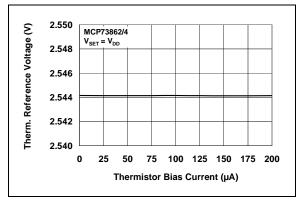
**FIGURE 2-21:** Thermistor Reference Voltage (V<sub>THREF</sub>) vs. Thermistor Bias Current (I<sub>THREF</sub>).
