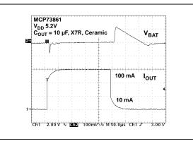
FIGURE 2-26: Load Transient Response.
