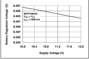
**FIGURE 2-14:** Battery Regulation Voltage (V<sub>BAT</sub>) vs. Supply Voltage (V<sub>DD</sub>).
