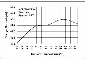
**FIGURE 2-32:** Charge Current ( $I_{OUT}$ ) vs. Ambient Temperature ( $T_A$ ).
