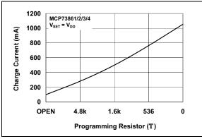
**FIGURE 2-31:** Charge Current  $(I_{OUT})$  vs. Programming Resistor  $(R_{PROG})$ .
