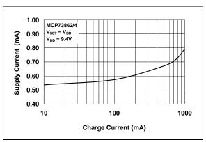
**FIGURE 2-16:** Supply Current ( $I_{SS}$ ) vs. Charge Current ( $I_{OUT}$ ).
