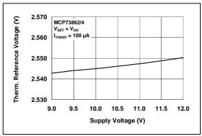
**FIGURE 2-20:** Thermistor Reference Voltage (V<sub>THREF</sub>) vs. Supply Voltage (V<sub>DD</sub>).
