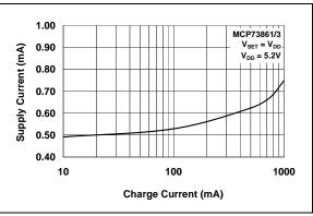
**FIGURE 2-4:** Supply Current ( $I_{SS}$ ) vs. Charge Current ( $I_{OUT}$ ).
