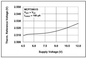
**FIGURE 2-8:** Thermistor Reference Voltage (V<sub>THREF</sub>) vs. Supply Voltage (V<sub>DD</sub>).
