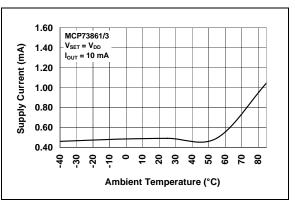
**FIGURE 2-10:** Supply Current  $(I_{SS})$  vs. Ambient Temperature  $(T_A)$ .
