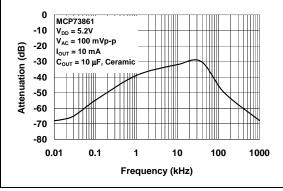
FIGURE 2-27: Power Supply Ripple Rejection.
