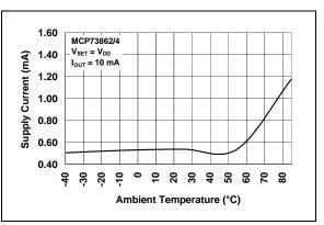
**FIGURE 2-22:** Supply Current  $(I_{SS})$  vs. Ambient Temperature  $(T_A)$ .
