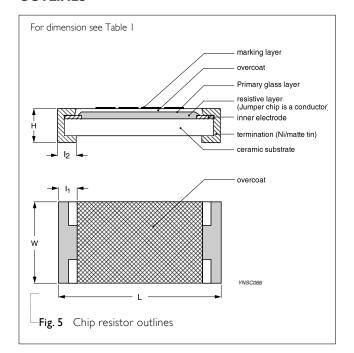
Chip Resistor Surface Mount RV SERIES 0603/0805/1206/2010/2512 (RoHS Compliant)
