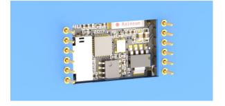
The IoD-09SM features surface mount castellated pads, and is designed to be soldered in place onto a host PCB. This module can be mounted on a PCB in 2 main ways.
