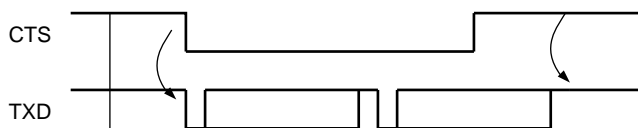
Figure 31-19. Transmitter Behavior when Operating with Hardware Handshaking
