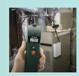
Check CO levels up to 999ppm with the push of a button using Model CO15. An audible alarm indicator will continuously beep starting at 25ppm (preset warning level - value can be adjusted) and the display will flash until the CO level goes down to normal range. A backlight on the display can be used for low light areas. The meter comes complete with batteries, wrist strap, and pouch.
