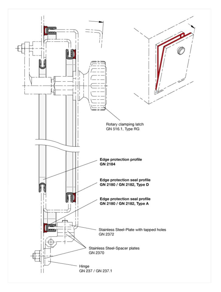
The construction depicted shows a standard application of edge protection profiles and edge protection seal profiles. The edge protection seal profiles are attached to the door and the fixed frame. The opening for the door is covered with an edge protection profile at its cut edge.
