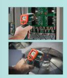
Compact non-contact InfraRed (IR) Thermometer measures up to 1112°F (600°C) with built-in laser pointer to identify target area and improve aim. Type K input allows for high temperature measurements up to 1832°F (1000°C). Builtin temperature sensor also measures Air Temperature. Adjustable emissivity feature allows for a higher accuracy when measuring temperature on various surfaces.
