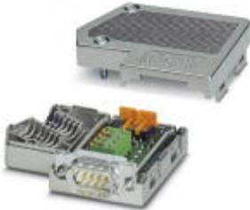
D-SUB plug, 9-pos., pin, axial version with two cable entries, below 35°, bus system: PROFIBUS DP up to 12 Mbps, termination resistor can be switched on via slide switch, pin assignment: 3, 5, 6, 8; spring-cage connection terminal blocks
