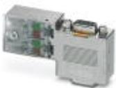
D-SUB connector, 9-pos., male connector, cable entry  $< 90^\circ$ , bus system: PROFIBUS DP up to 12 Mbps with PG D-SUB socket for connecting a programming device, termination resistor can be switched on via slide switch, pin assignment: 3, 5, 6, 8; IDC terminal block connection
