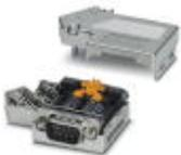
D-SUB connector, 9-pos., male connector, cable entry  $< 35^\circ$ , bus system: PROFIBUS DP up to 12 Mbps with PG D-SUB socket for connecting a programming device, termination resistor can be switched on via slide switch, pin assignment: 3, 5, 6, 8; screw connection terminal blocks
