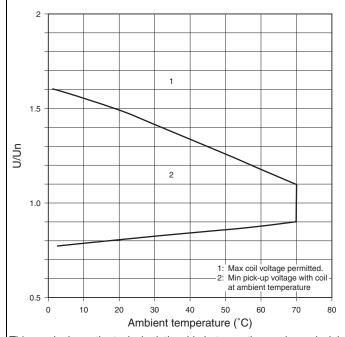
This graph shows the typical relationship between the maximum / minimum coil and pick-up voltage and ambient temperature
