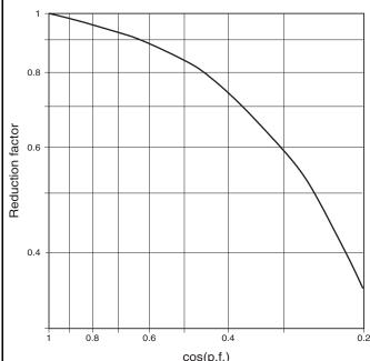
For AC inductive loads (such as solenoids, contactors coils, etc.) the reduction factor corresponding to cos(p.f.) (cosine of the power factor) is multiplied by the rated current in order to identify the maximum allowable current. This approximation is not valid for loads with high inrush currents such as electric motors or fluorescent lamps.
