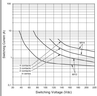
This graph can be used to estimate the number of contacts that can be used to switch DC resistive loads
