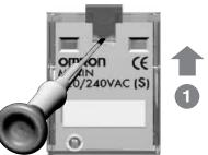
Push up the test button to the first position, then press the yellow button with an insulated tool to operate the contact.
