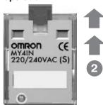
Push up the test button to the second position. (The contact is now in the locked position).
