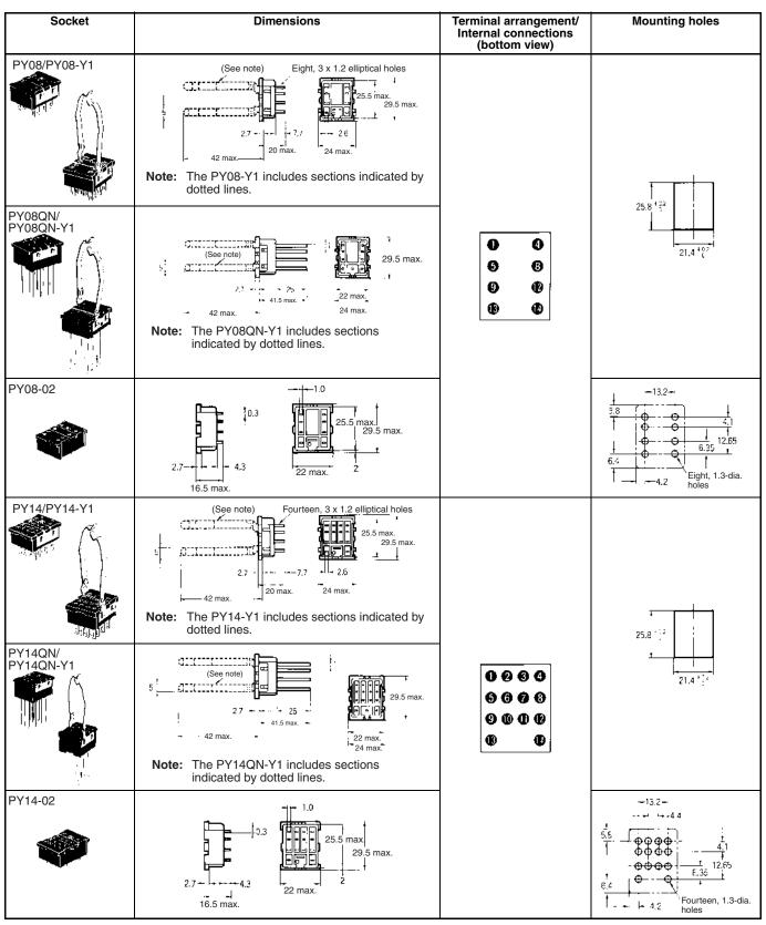
Note: Use a panel with plate thickness of 1 to 2 mm for mounting the Sockets.
