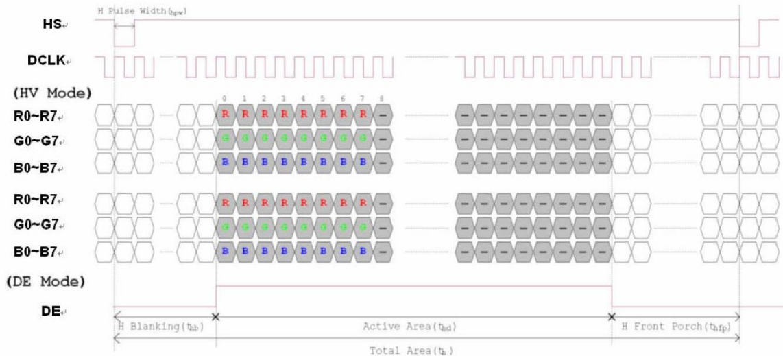
Figure 7. Horizontal input timing diagram
