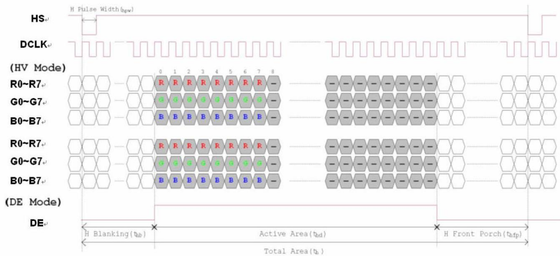
Figure 7. Horizontal input timing diagram
