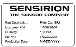
**Figure 4:** Label on shipment packaging: Customer P/N refers to the Sensirion product number, Lot No. refers to suppliers tracking information. Production Date is given as MM = month, DD = day, YYYY = year.
