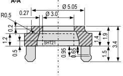
**Figure 1:** Drawing of the Filter Cap SF2 (body only). Dimensions are given in mm (1mm = 0.039inch), tolerances are  $\pm 0.1$ mm. Add 0.15 to total height due to the filter membrane. The cavity inside the cap fits to SHT2x sensors. Additional space for solder joints are left open around the sensor.
