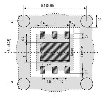
**Figure 3**: PCB layout of SHT2x and Filter Cap SF2. Dimensions are given in mm (1mm = 0.039 inch). The distance of the openings is  $5.1 \text{ mm} \pm 0.05 \text{ mm}$  if the sensor should clip on the PCB and 5.28 mm if the pins are used for adjustment only. By varying the openings distance about  $\pm 0.05 \text{ mm}$  the cliping force may be adjusted.
