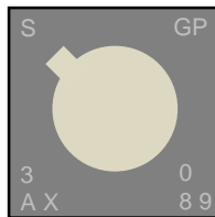
Figure 10 Laser marking on SGP30. The pin-1 location is indicated by the keyhole pattern in the light-colored central area. The bottom line contains a 4-digit alphanumeric tracking code
