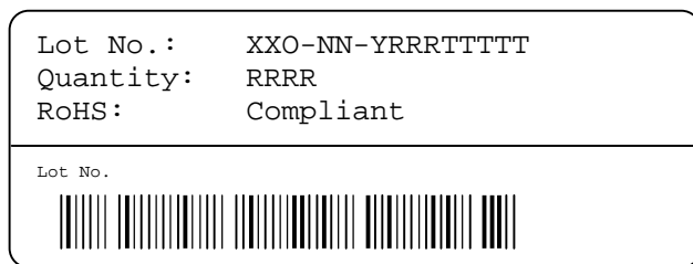
Figure 13: First label on reel: XX = Sensor Type (21 for SHT21), O = Output mode (D = Digital, P = PWM, S = SDM), NN = Chip Version, Y = last digit of year, RRR = number of sensors on reel divided by 10 (200 for 2000 units), TTTTT = Traceability Code.
