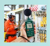
Extech's ultra-compact sound meter meets class 2 standards with ±1dB high accuracy that allows for quick and reliable sound level testing. It features a large backlit display for easy viewing and measures A & C weighting from 35 to 130dB with Fast and Slow response time mode. Size is small enough to conveniently fit in your pocket and includes a wrist strap.
