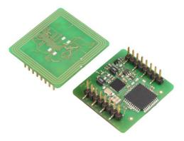
Elatec's Mini Reader MIFARE NFC is designed for integration into machines, handheld computer or any other device. The focus has especially been set on size, low power, price and flexibility. Thanks to its compact dimensions, integration directly on a PC board is possible.
