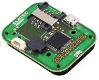
TWN4 MultiTech 3 HF PCB top view
