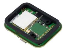
TWN4 MultiTech 3 HF PCB bottom view
